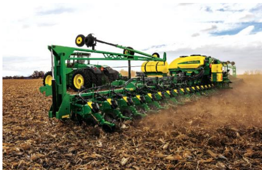
Figure 19. Typical conservation tillage planter.
