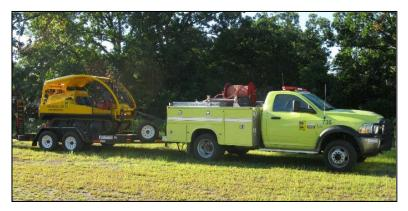
Type 6 engine towing J-5 tracked vehicle
