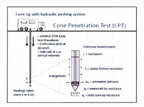
Figure 7 Schematic view of the piezocone
