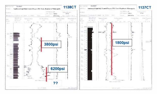
Figure 11 Soil strength variability from CPT borings.
