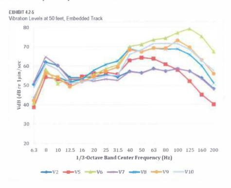
Figure 3 Estimated vibration levels 50 feet from an at-grade source.
