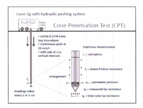
Figure 7 Schematic view of the piezocone
