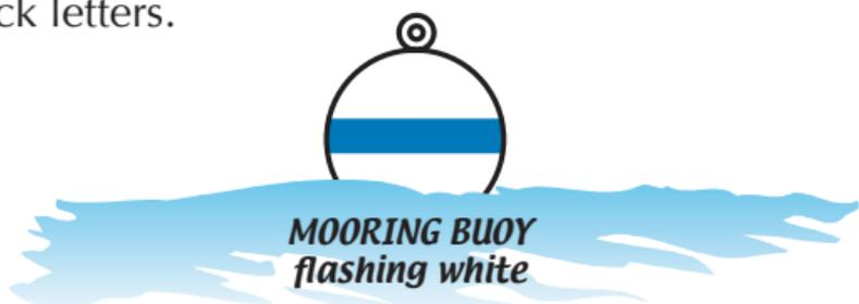
★ **Mooring Buoys.** Buoys designed for mooring boats are all-white with a blue stripe midway between the top and the waterline. A minimum of 16 square inches of white reflectorization, part of which must be visible from any direction, is required on all mooring buoys. (Obtain a permit from the county sheriff before placing a mooring buoy in the water.)
