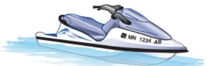
What is a personal watercraft? Sometimes known as **Jet Skis, Wave Runners, Sea Doos**, water scooters etc., a personal watercraft is defined by law as a motorboat that is: 1) powered by an inboard motor powering a water jet pump or by an outboard or propeller-driven motor; and 2) designed to be
