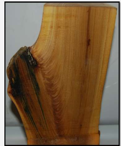
Figure 60. CODIT as dark color in plugged vascular tissue..
