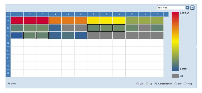
Figure 5. A heat map of samples that were previously analyzed and were questionable in regards to being positive for H. irregulare. A new analysis shows rows A (wells 1 to 12) and B (wells 1 to 3) of positive controls amplifying at known concentrations. High con
