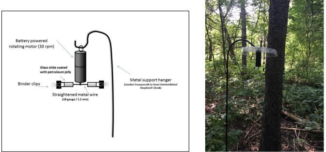
Figure 8. Diagram of a spore sampler showing the different parts that compose the sampler (left). Spore sampler that has been placed in Minnesota (right).
