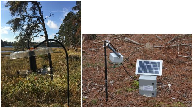
Figure 9. Spore sampler in Itasca State Park (left). A new spore sampler being tested contain two small rods that are programmed to spin at specific time intervals and collect airborne spores. This sampler (right) appears to be more sensitive and efficient at collecting the very small spores produced by Heterobasidion.
