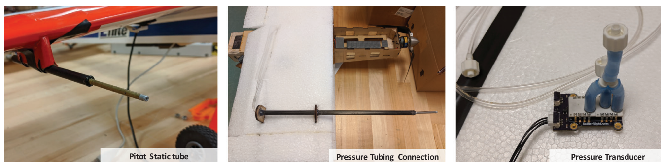
FIGURE 2 Entire ADS using a pitot-static tube, pressure tubes, and a pressure transducer for a small UAS [Color figure can be viewed in the online issue, which is available at wileyonlinelibrary.com and www.ion.org ]
