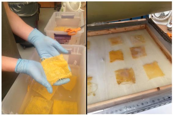
Fig. 14 Picture of the design of floating biofilm in wastewater for nutrient recovery
