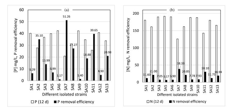
**Fig. 3** Nutrient removal efficiency [a. Phosporous recovery b.Nitrogen recovery] of the different isolated fungi from sarita wetland
