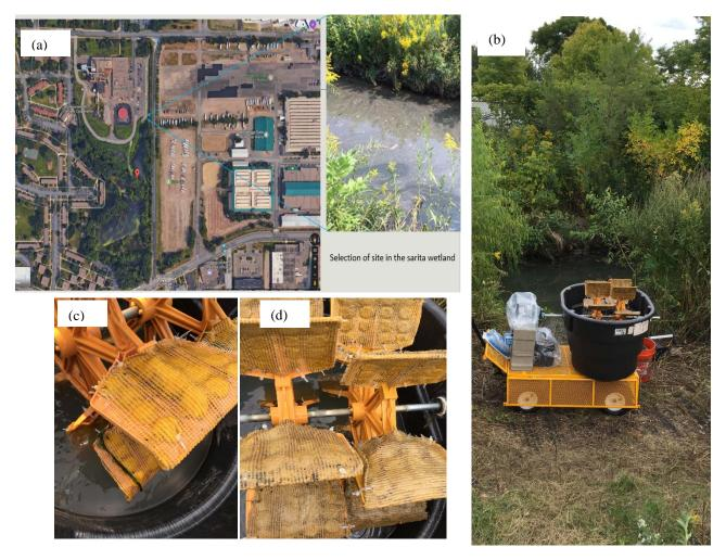
**Fig. 18** (a) Location of the Sarita wetland (b) Paddle wheel reactor onsite for the nutrient recovery (c) Biofilm on the paddle recovering P,N and COD in Sarita wetland and the (d) biofilm after 7 days of
