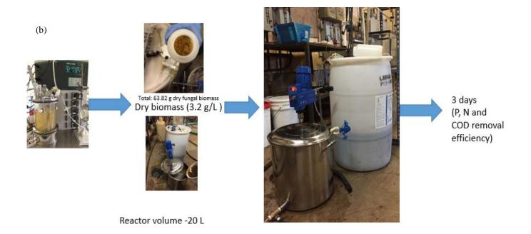
Fig. 19 (a) Schematic representation of the biofilm reactor for nutrient recovery from manure water and (b) prototype model
