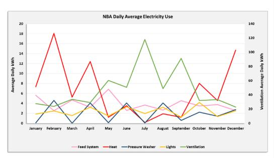
Figure A15. The monthly averages of daily energy use by various electrical loads measured at NBA from January 2015 to March 2017. No data is estimated.
