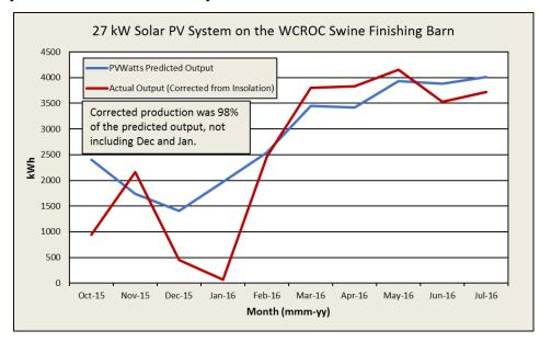
Figure 12: Corrected electricity production from the WCROC solar PV system.
