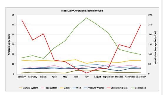
Figure A21. The monthly averages of daily energy use by various electrical loads measured at NBB from January 2015-March 2017.
