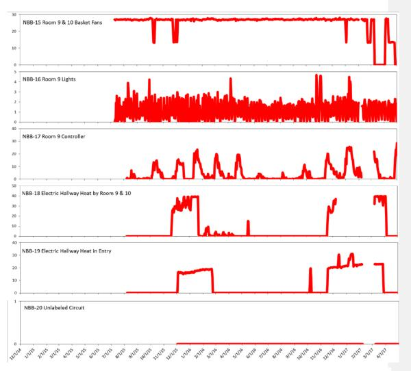
Figure A19. Timeline of sensors from beginning of installation to end. Gaps in data represent areas where data was lost due to battery issues or unplugged cables. All data is in kWh.
