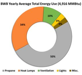
Figure A12. The total average energy use averaged across 2015 and 2016 and converted into MMBtu across several larger electrical loads and propane consumption in BWB. (1 kWh=3412.14 btu. 1 therm= 91.600 btu)
