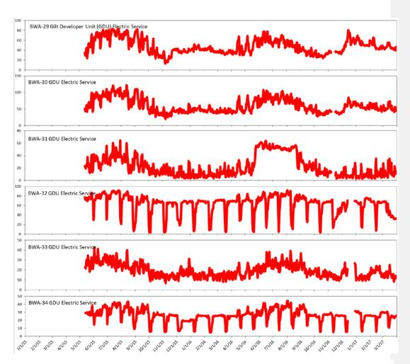
Figure A1. Timeline of sensors from beginning of installation to sensor and data logger removal. Gaps in data represent areas where data was lost due to equipment failure. All data is in kWh.
