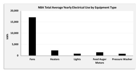
Figure A16. The average yearly electricity use (2015-2016) by equipment type in NBA.
