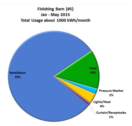
Figure 9. Example breakdown of energy used for processes within a cooperator swine facility
