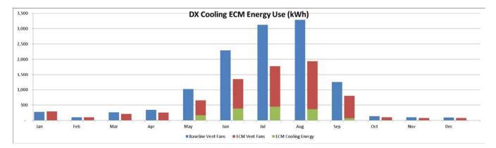
The DX air conditioning system has a similar effect on the finishing barn while showing greater fan power savings.
