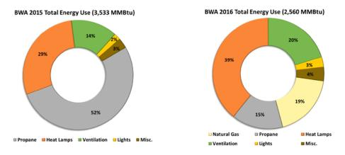
Figure A6 and A7. Total energy use converted into MMBtu across several larger electrical loads and propane/natural gas consumption in BWA in 2015 and 2016. (1 kWh= 3412.14 btu, 1 therm= 91,600 btu)
