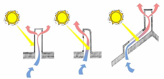
Solar/thermal chimneys use the sun's heat to increase the stack effect drawing air out of the barn. A solar chimney could be sized to induce outdoor air into the barns without the use of fans. Ventilation is required 24 hours per day, so fans would still be required to supplement and back up the flow of the chimney when there is not sufficient temperature differential between the interior space and the chimney to maintain flow.
