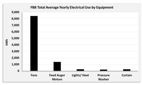
Figure A32. The average yearly electricity use (2015-2016) by equipment type in FBB.
