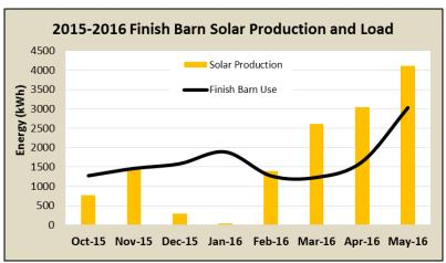
As it was predicted early on in the project, the solar array will produce the most energy during the summer months, when solar radiation is highest. The predicted increased production can be observed beginning earlier this spring and is well matched to the increasing load due to expanded use of ventilation fans to cool the pigs.
