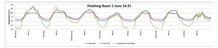
While traditional air conditioning has a positive effect on stabilizing and lowering the peak indoor temperatures of the barns as well as reducing the required fan power, there is very little savings in energy cost or energy use. This equates to long payback periods that do not justify this ECM unless the goal is to provide better thermal comfort for the pigs which may have positive results in health and growth.
