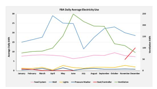
Figure A26. The monthly averages of daily energy use by various electrical loads measured at FBA from January 2015 to March 2017. It should be noted that there were data logger battery issues during both years that resulted in some data lost for "Heat/Controller" from July to October. The data that was available is reflected in this figure and no missing data was estimated.
