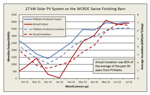
Figure 11: Actual electricity production from the WCROC solar PV system and average monthly insolation from the pyronometer at the WCROC weather station compared with predicted output and insolation from PVWatts.
