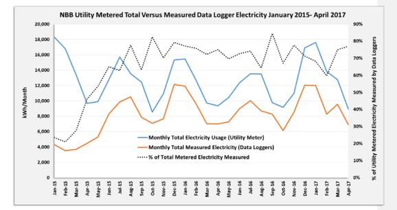
Figure A20. Total monthly electric usage of NBB as obtained from the facility's electric bill, the total monthly amount of electric usage captured by installed data loggers and sensors, and the percent of electricity measured compared to the metered total. As additional data loggers were added to this facility, the percentage of electricity captured by loggers can be seen to increase.
