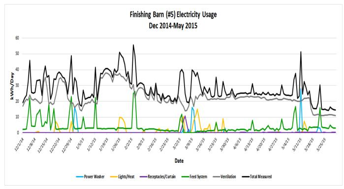
Figure 8 Example of weekly energy usage data from a cooperator swine facility
