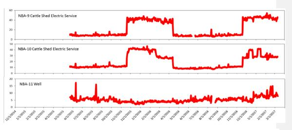
Figure A13. Timeline of sensors from beginning of installation to sensor and data logger removal. Gaps in data represent areas where data was lost due to battery issues or unplugged cables. All data is in kWh.
