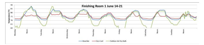
These charts show the effect of converting the full heating load over to the geothermal system as well as adding cooling. The result is a large reduction in total energy use as the primary benefit.
