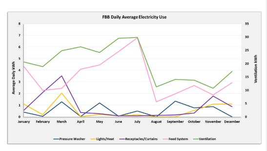
Figure A31. The monthly averages of daily energy use by various electrical loads measured at FBB from January 2015-March 2017. It should be noted that there were data logger battery issues during both years that resulted in some data lost for "Feed System" in January and from August to November and from "Ventilation" from August to November. The data that was available is reflected in this figure and no missing data is estimated.
