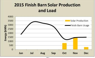
(minus the missing data) compared to the electricity actually used in the finish barn during the same time frame. The finish barn electrical usage is from a utility meter dedicated to the finish barn.
