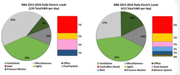
Figures 8 and 9. The average daily electricity use across electrical loads in NBA and NBB.
