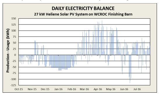
Figure 9: Amount of excess electricity produced from the WCROC solar PV system.
