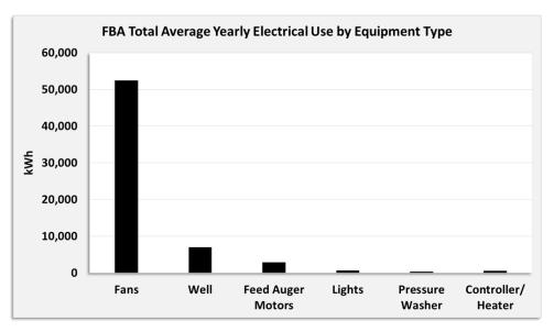
Figure A27. The average yearly electricity use (2015-2016) by equipment type in FBA.
