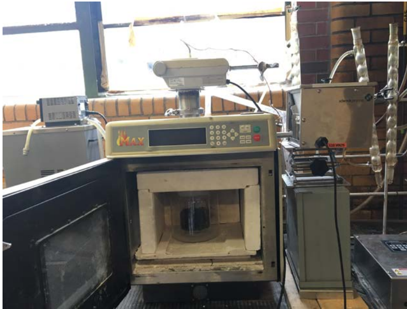
Fig. 2 The lab-scale continuous microwave based system
