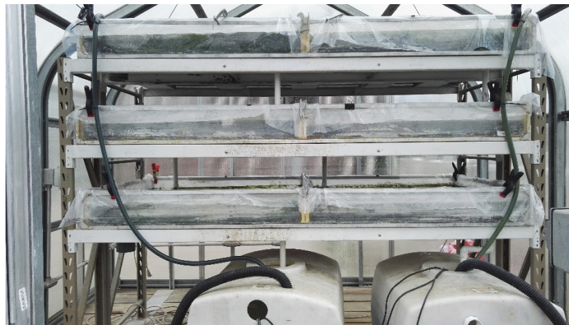
Figure 1. Two PBRs system at the Metro Plant.
