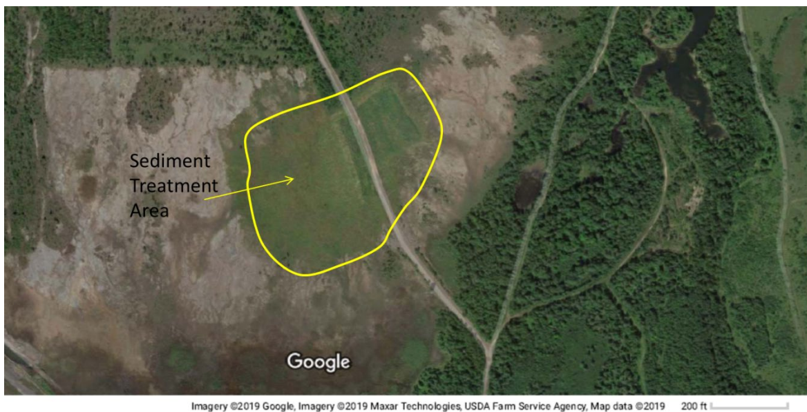
Figure 3-10: 2019 KeeTac project site about 8 years after sediment application. Green edge of the vegetation is associated with the extent of sediment application.
