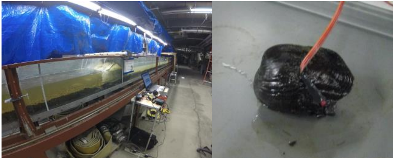
Figure 2. Flume setup for testing mussel response to suspended sediment. Gape sensors (right) will be attached to mussels to measure filtering response as a function of suspended sediment load.
