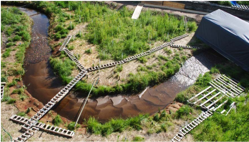
Figure 8. Mussel response to bed instability was observed in the Outdoor StreamLab at SAFL. Mussel movement was tracked using unique identifiers.
