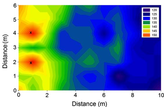
**Fig. 2** The sound intensity level (dB re 1  $\mu$ Pa @ 1 m) is plotted during active broadcast of the two underwater speakers (indicated by X). Recordings were made at 1 m intervals and a depth of 0.6 m. Intensity level is indicated by color in upper right inset
