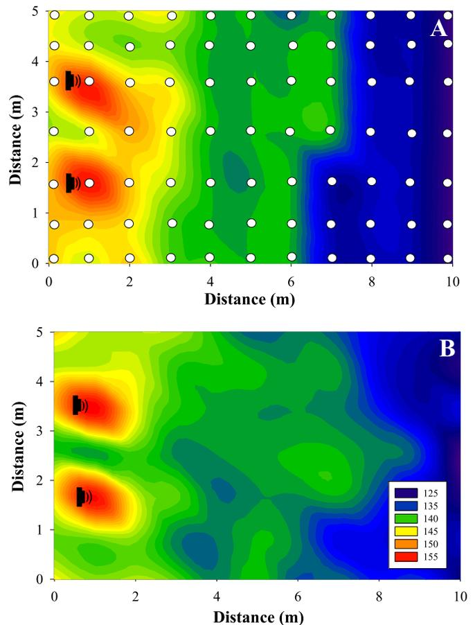
**Fig. 1.** Sound pressure level in the experimental pond. The sound intensity was measured using a hydrophone at a depth of 0.6 m at 77 intervals throughout the pond during broadband sound playback. The speakers and points of measurement (white circles in upper figure) are indicated. The colors represent the sound intensity level (dB re 1  $\mu$ Pa), indicated in the scale on the lower right. A) 1000 Hz pure tone; B) Broadband sound stimulus.
