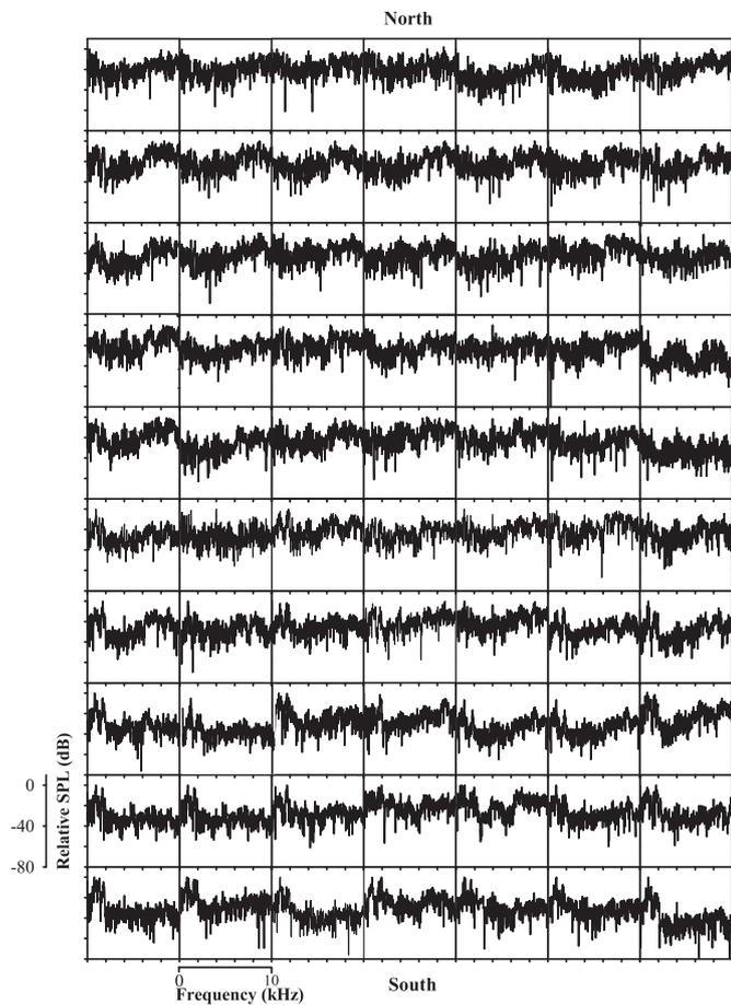
**Fig. 3.** The power spectrum from measurement locations in the pond is plotted versus frequency during playback of the broadband sound. The maximum sound pressure level at each location was assigned a decibel level of 0 and each spectrum is plotted relative to the maximum sound pressure level at each location.
