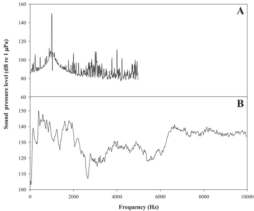
**Fig. 2.** The power spectrum of the A) pure tone (1000 Hz) and B) broadband sound is plotted versus frequency from a hydrophone a depth of 0.6 m directly in front of the speaker (<1 m) during sound playback in the pond (Modified from Vetter et al., 2015).
