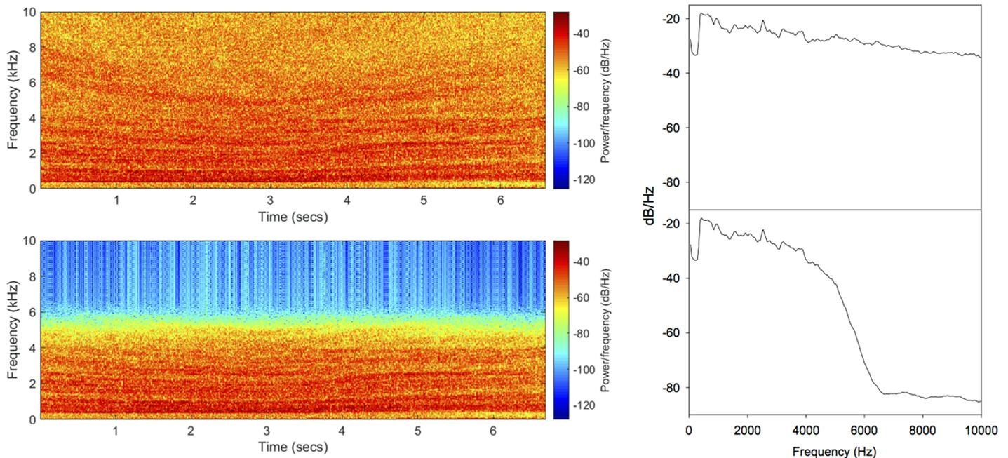
**Fig 7. Low-pass filtered broadband sound.** Spectrogram (left) and power spectrum (right) of the unfiltered (top) broadband sound used by Vetter et al. [14, 15] and Murchy et al. [10] to deter bigheaded carp. Bottom spectrogram and power spectrum represent the same broadband sound with a 5 kHz low-pass filter applied using Audacity (version 2). Spectrograms were generated using MatLab (version 9.3) and power spectra were analyzed in Audacity.
