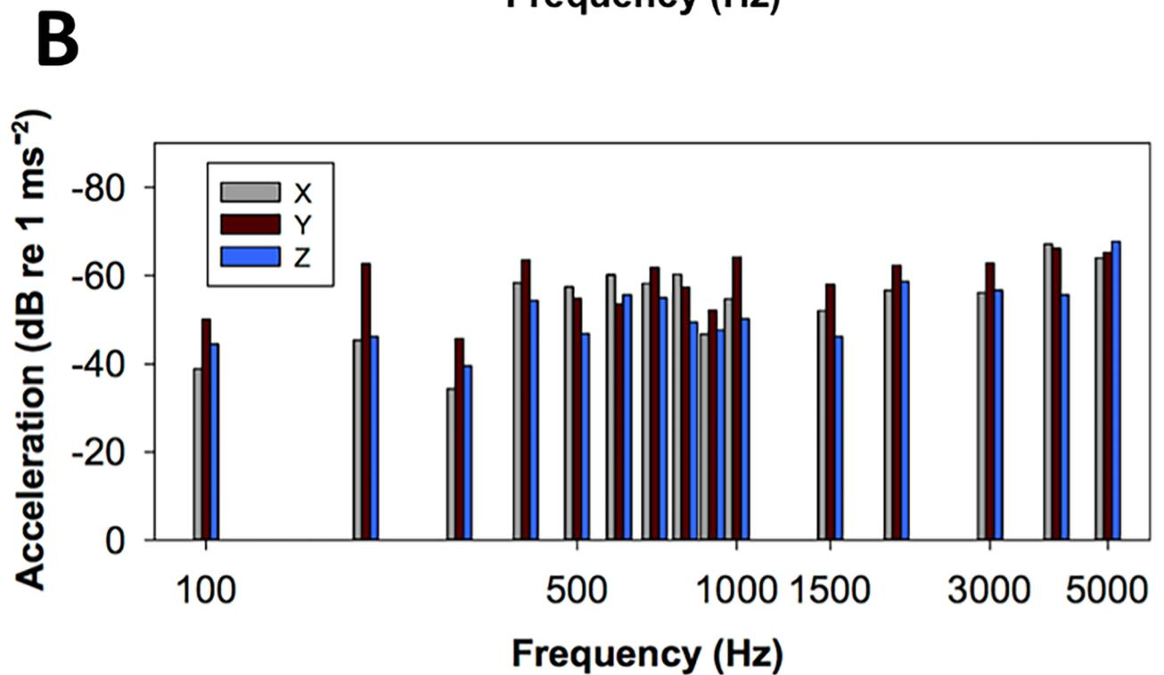
**Fig 1. Acoustic characterization of the experimental tank.** A) Acoustic impedance (ratio of sound pressure level to particle motion level) at three sound pressure levels (119, 130, and 145 dB  $1 \mu\text{Pa SPL}_{\text{rms}}$ ) for all frequencies examined. There are no apparent resonances at any of the frequencies. B) Particle acceleration levels for each of the x, y, and z magnitude vectors at 130 dB re  $1 \mu\text{Pa}$  for all frequencies examined.
