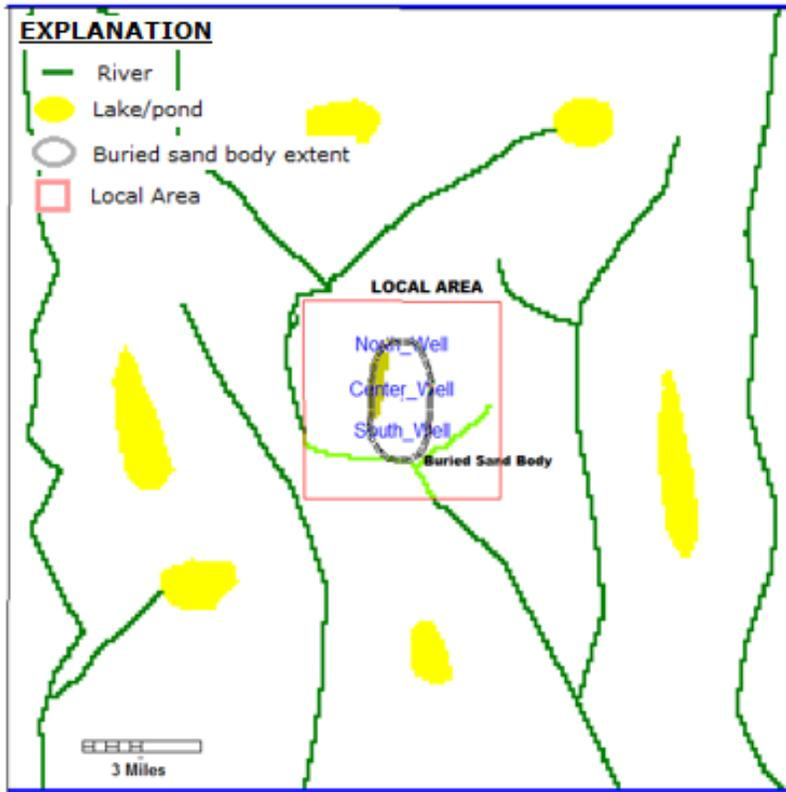
Figure 5. Aerial view of the base conceptual groundwater-flow model.
