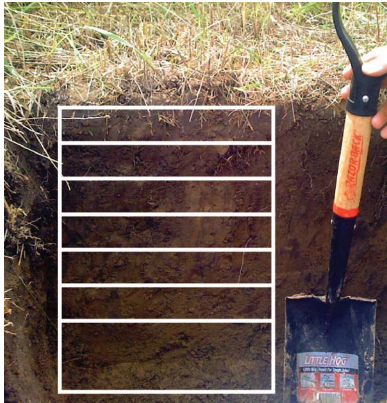
Figure 2. Photo showing sample collection increments for a typical soil pit. Pit face sampling was performed for the upper 50 cm. A multi-stage core sampler was used to collect samples to a depth of 150 cm.
