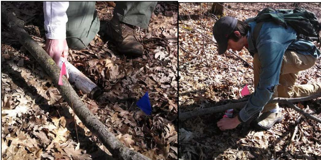
Figure 25. Incubation tubes (short lengths of PVC tube) were hammered into the ground, capped and left in place for 28 days.
