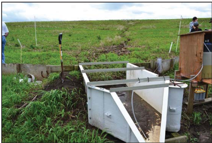
Eroded soil frequently needs to be cleaned out of the testing flue in the left photo, even though the cropped acres above it are in a no-till system. The flue in the right photo, which sits at the base of a field plot's native prairie strips, is virtually free of eroded soil. "I was shocked at how much soil was being lost," says farmer Gary Van Ryswyk of the field plot without prairie. (LSP photos)
