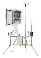
To improve fire weather forecasting and preparedness, several Remote Automatic Weather Stations (RAWS) received modification to the new Tri-leg format. This allows for easier maintenance and location changes if necessary. There are still 37 RAWS in Minnesota used for fire danger predictions and monitoring.
