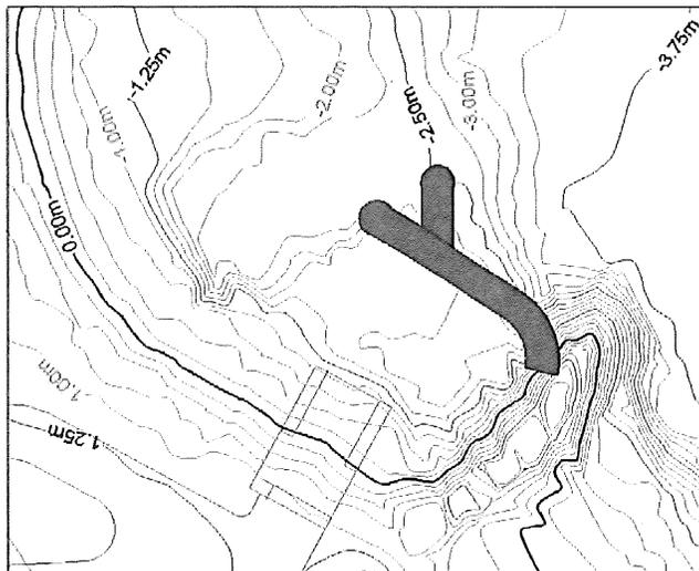
Figure 21 Alternative 2: Fishtail Breakwater
