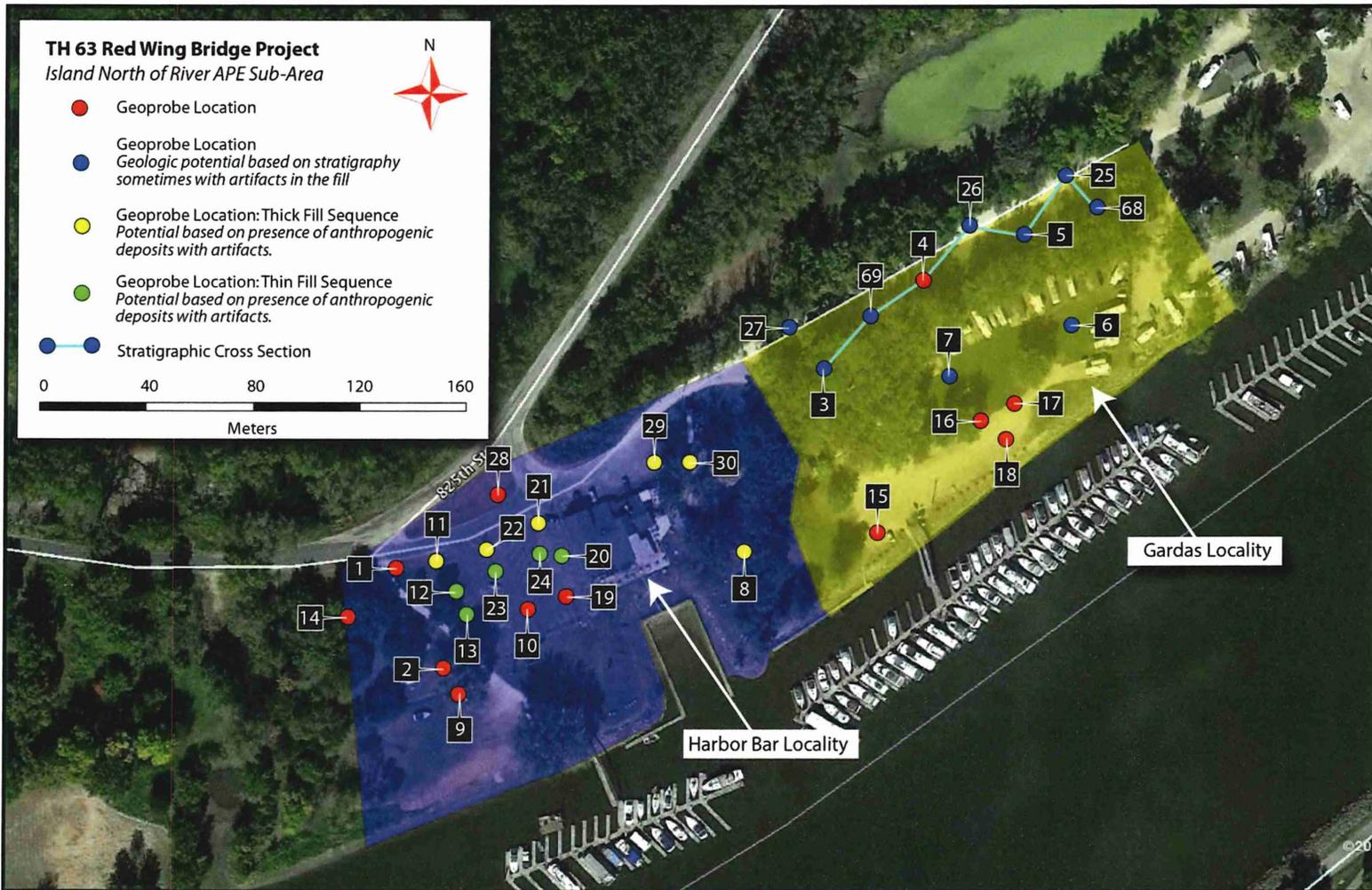
Figure 3. North of the River Subarea core locations & geologic potential
