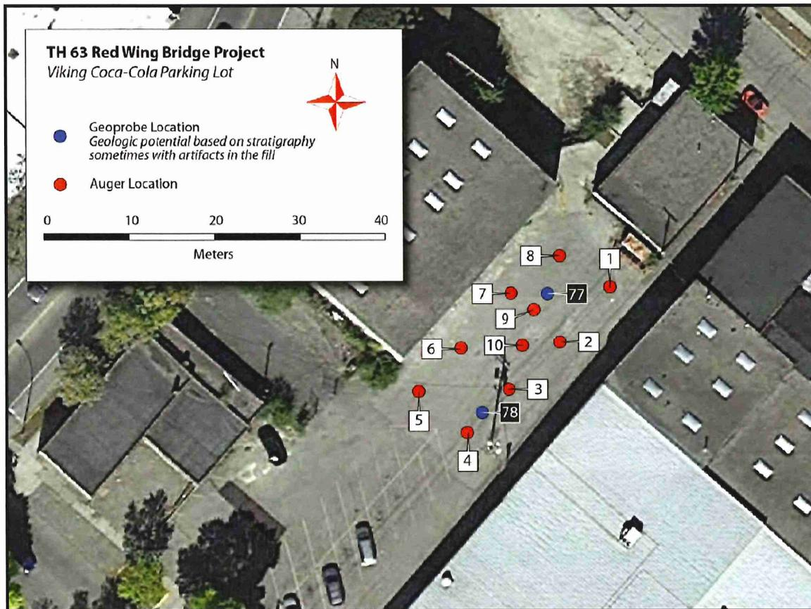
FIGURE 40. PLAN OF GEOPROBE CORES WITHIN AREA 25 (KOLB 2014:27)
