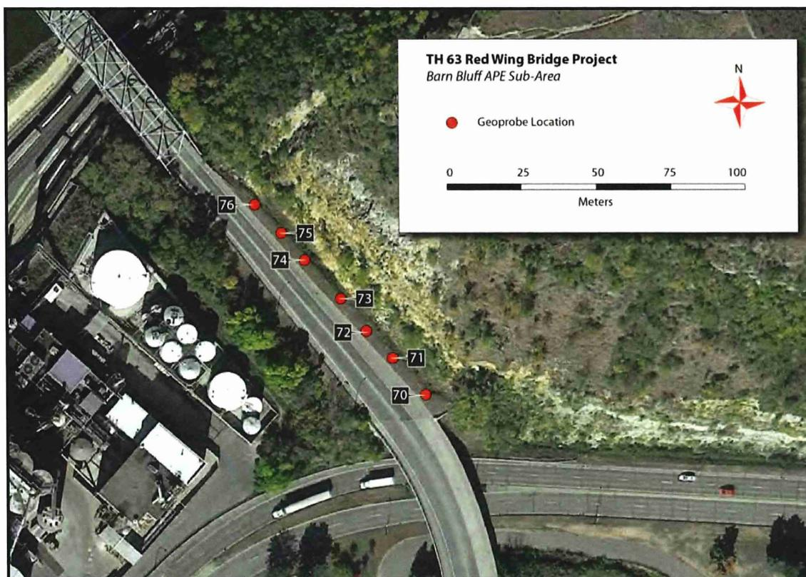
FIGURE 60. PLAN OF GEOPROBE CORES WITHIN THE BARN BLUFF SUB-AREA (KOLB 2014:33)
