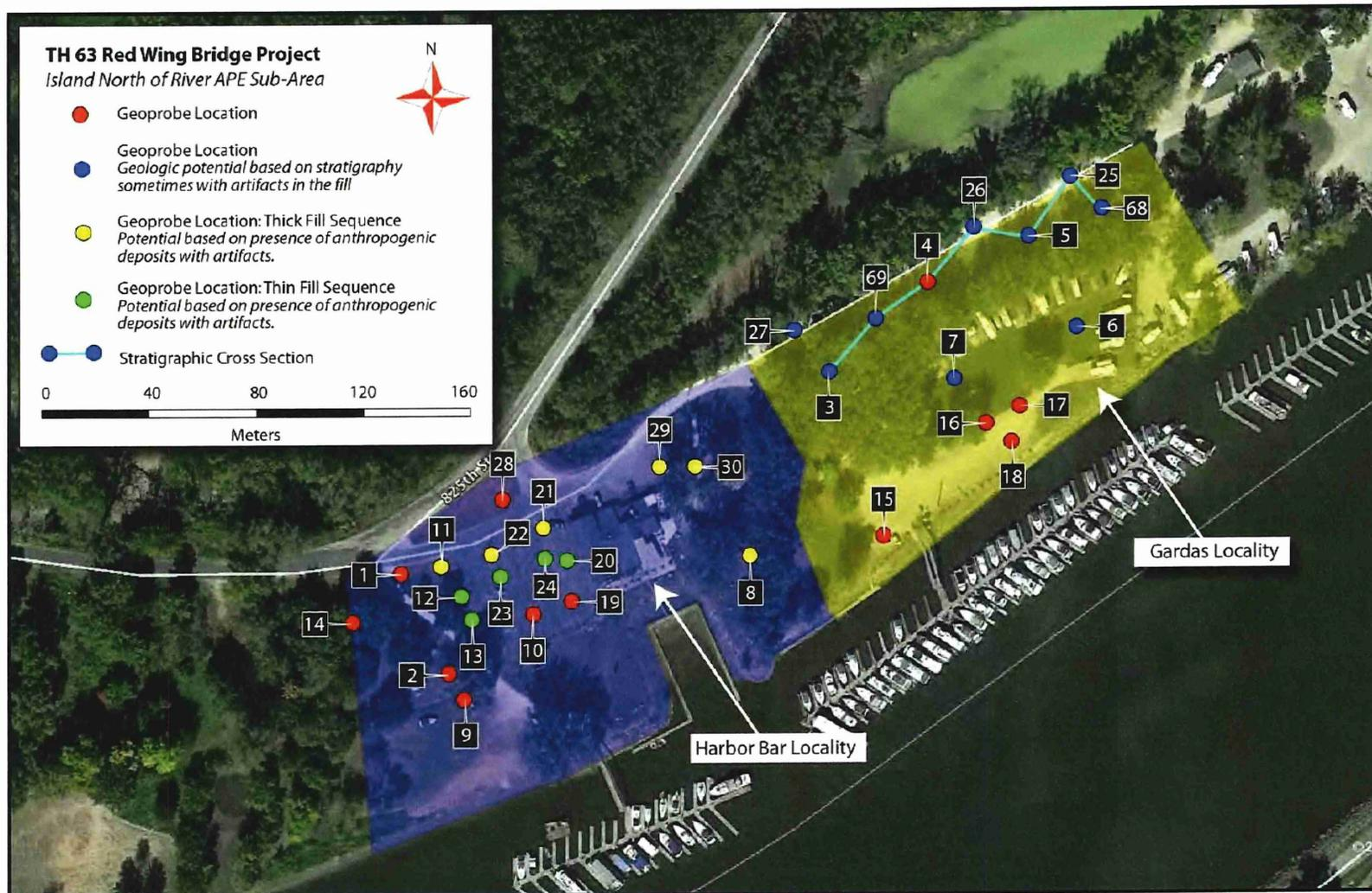
FIGURE 15. PLAN OF GEOPROBE CORES WITHIN THE NORTH OF THE RIVER SUB-AREA (KOLB 2014:6)
