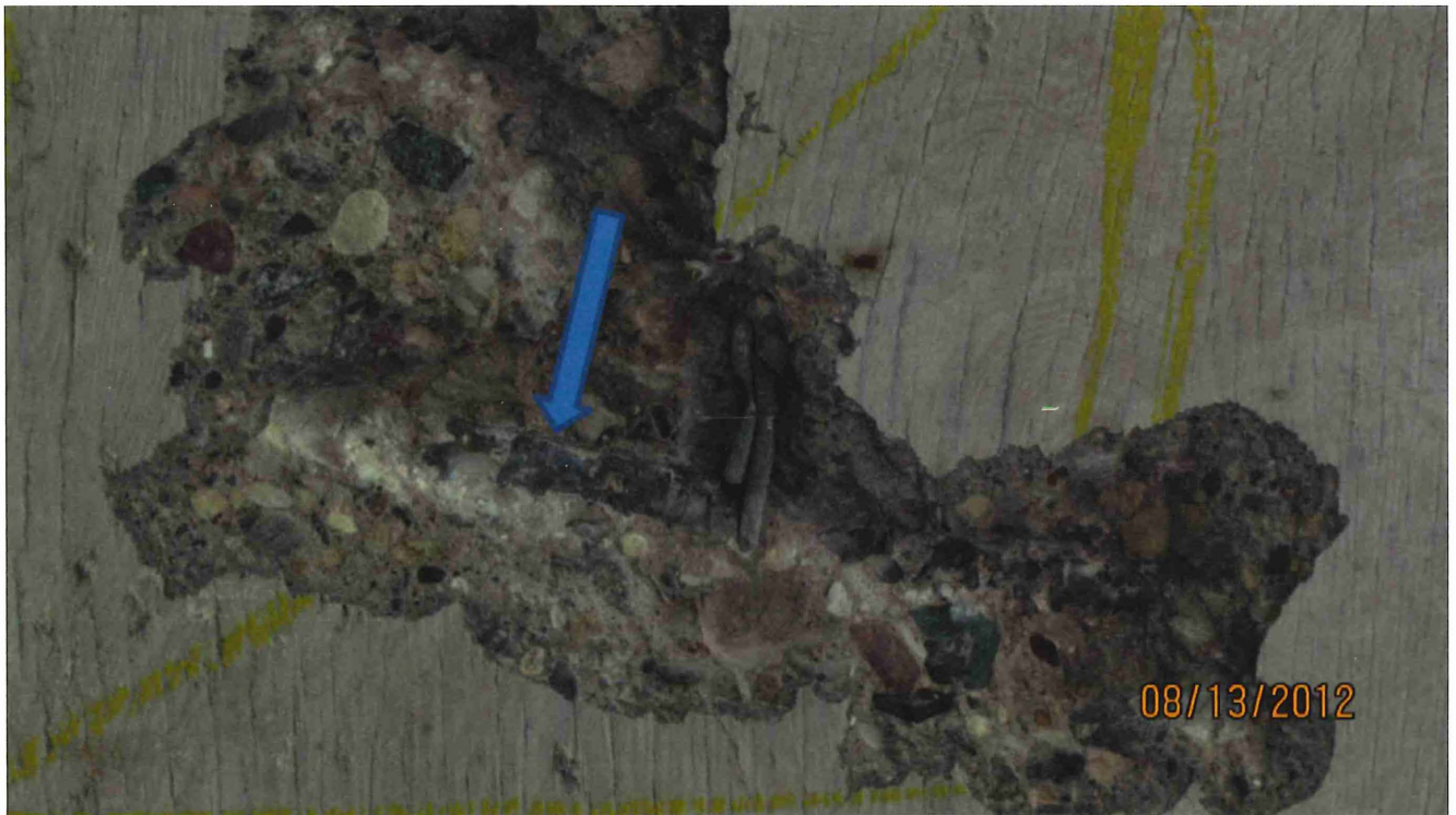
Sample # 4 after concrete has been removed. Rebar shows no sign of rust.
