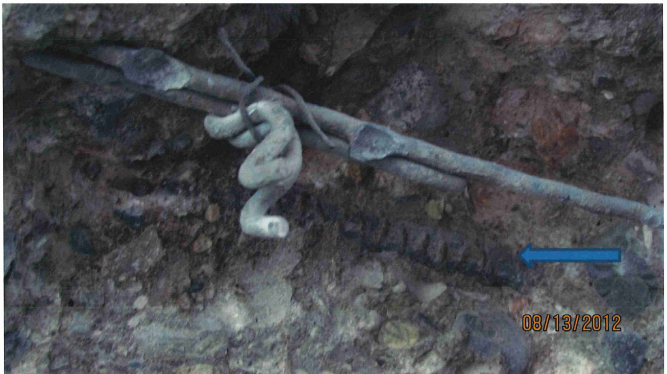
Sample # 3 after removal of concrete no rust or rust staining. This was in the area of highest chloride concentrations near the full depth core.
