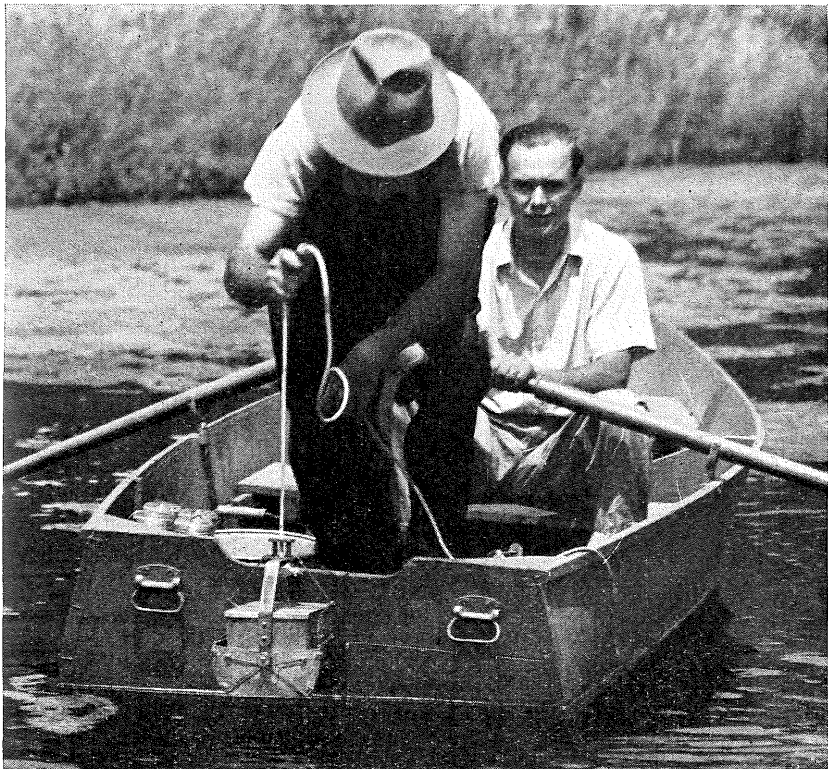
The small sized dredge brings up samples of lake bottom soils for study.
