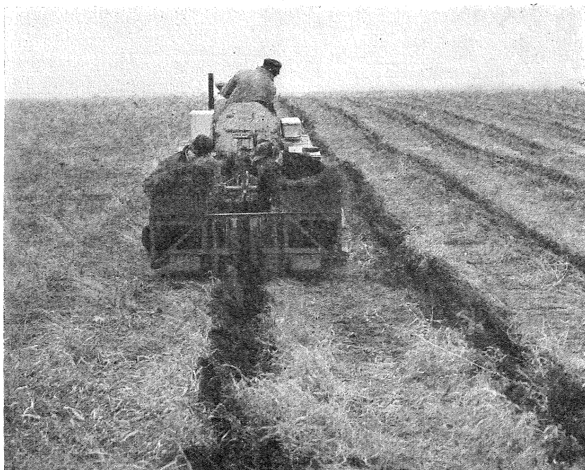
Two men sit in rear of tree-planting machine and alternately feed trees through center slot.
