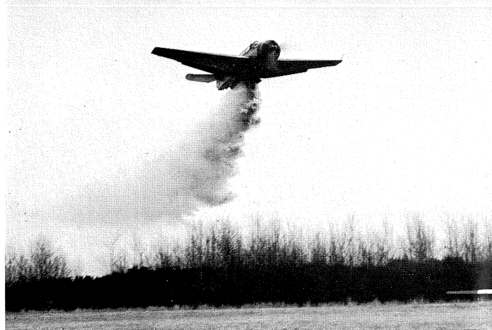
FIGHTING FIRES — Via aerial assault, a converted Navy torpedo bomber (TBM) jettisons a load of fire retardant chemicals during the course of a "test run" in the Grand Rapids area. Trials of this modern-day fire fighting procedure have proved so promising the Department of Conservation has slated more intensive testing of the technique.—Cut courtesy Grand Rapids Review.
