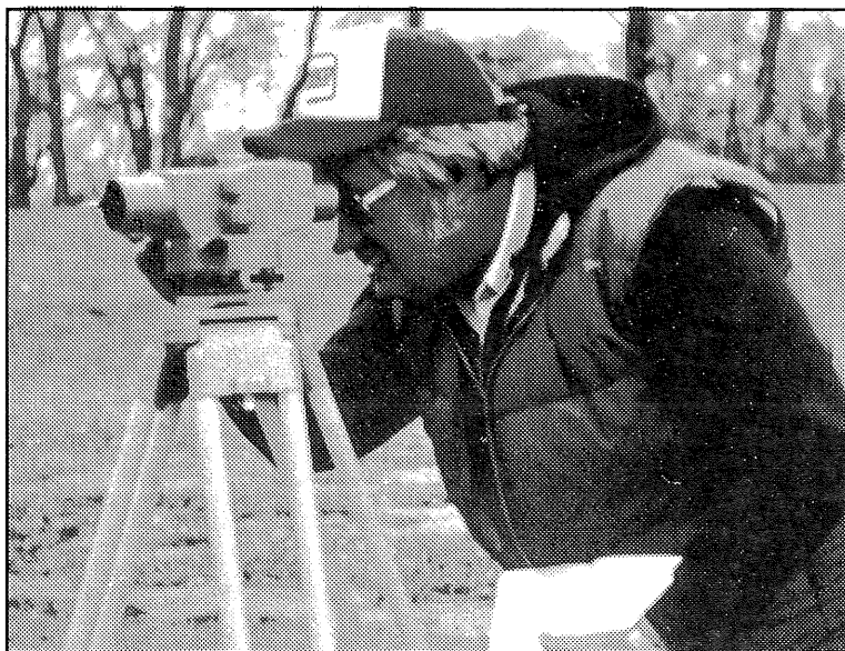
Figure 3.3 Cross section data are usually obtained by field surveys.
