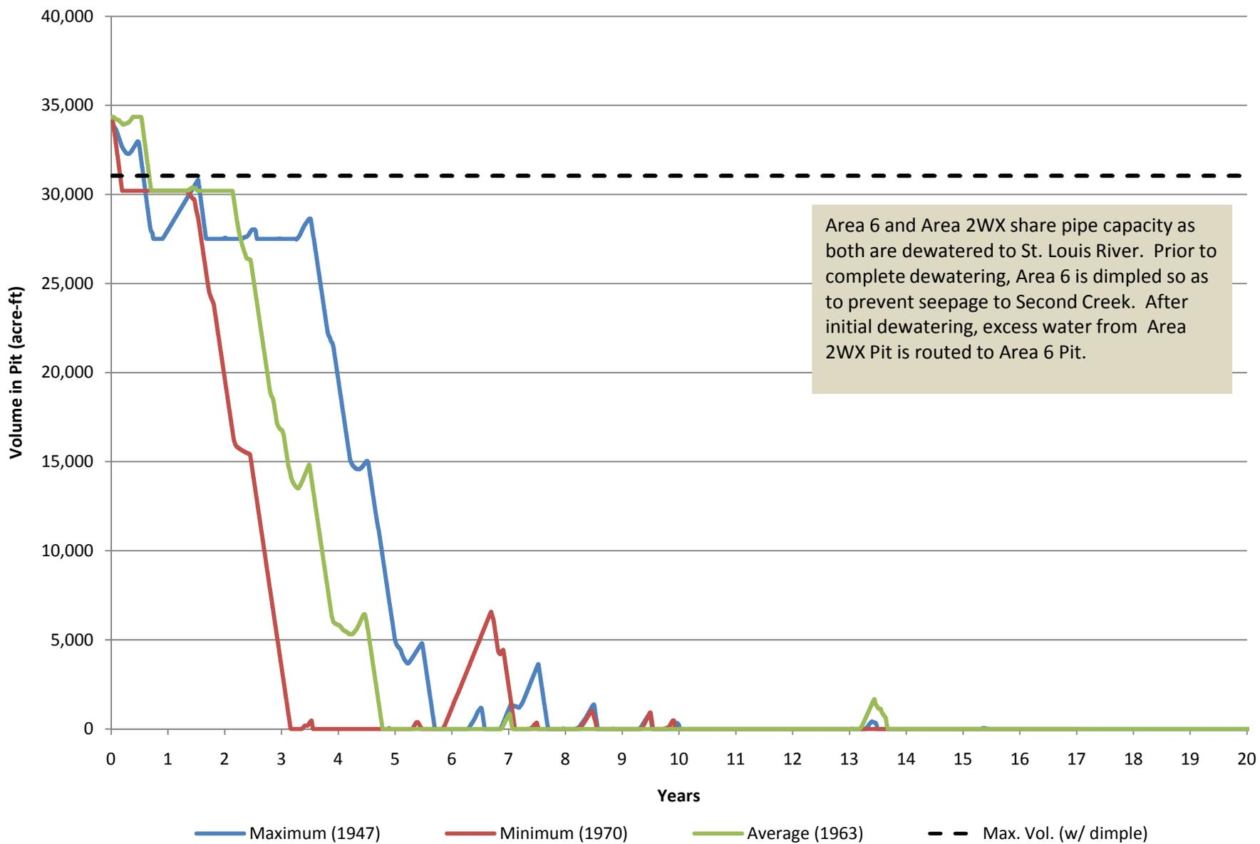
**Figure 5. Volume of Water in Area 2WX Pit during Mining Alternative 1**
