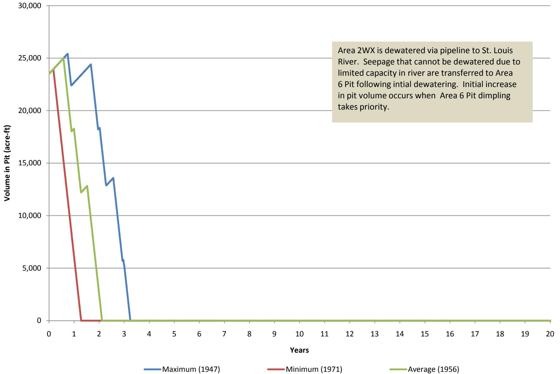
**Figure 6. Volume of Excess Water In Area 1 Pit during Mining Alternatives 1 and 2**
