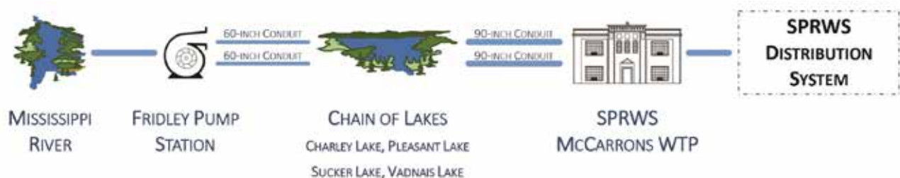
Figure 3-1. Schematic of SPRWS Raw Water and Treatment Infrastructure.
