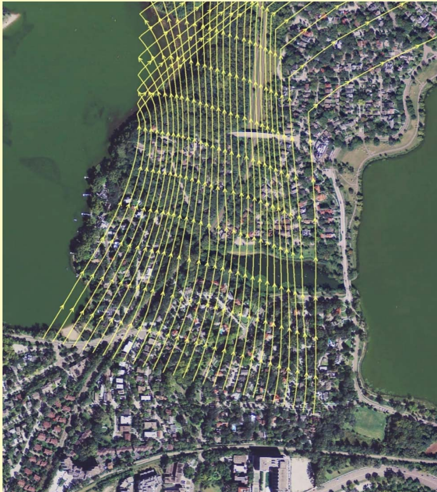
Shallow groundwater flow direction
