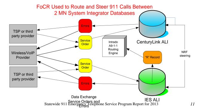
As illustrated in the diagram above, because two different legacy 911 System Integrator's location databases operate in the state of Minnesota an application call Function of Code R (FoCR) is required. This application enables the location and telephone number to move across the ESInet so that PSAPs can transfer calls with location information as well as the 911 call can be delivered to the correct PSAP. This functionality provides a faster and more assured response for the 911 caller.
