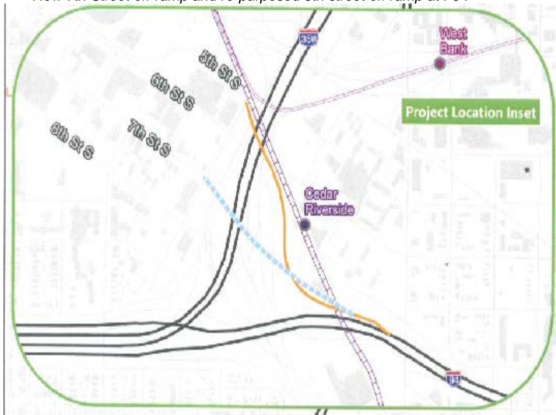
New 7th Street off-ramp and re-purposed 5th street off ramp at I-94
