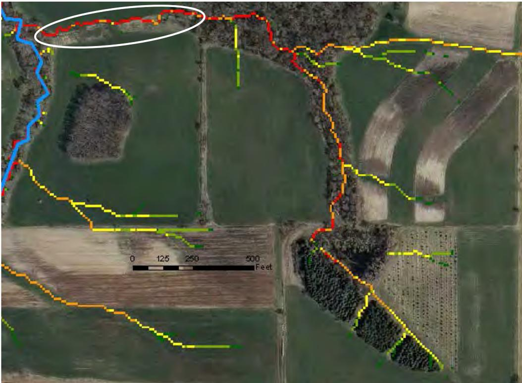
The image on left shows a long (~1/2 mile) SPI signature with several high SPI values following a forested ravine. Users would typically expect to see surface erosion associated with such an SPI, though a field visit showed very little erosion and soil deposition evident from the upslope tree line to the pour point due to a well maintained filter strip (circled in white).
