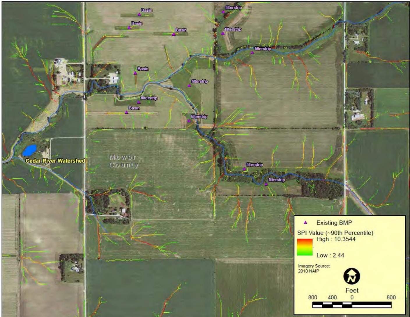
For the same area, the following figure shows the delineated area tributary to each of the remaining CSAs. The resulting drainage areas for each CSA can be intersected with the watershed modeling output to further prioritize potential project areas following field verification of the delivery mechanisms and/or erosion potential.
