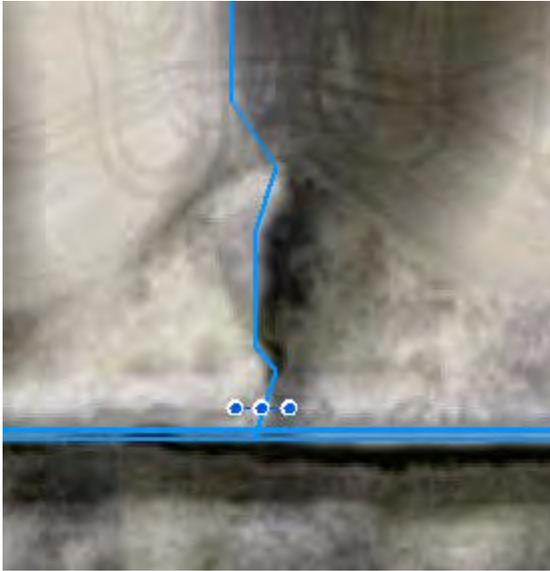
The blue stream line oriented north-south in the image on left is flowing south and empties into the east-west oriented stream. To create a catchment of the north-south stream, a digitized outlet (shown with blue dots) is made perpendicular on that stream near its outlet. The catchment will terminate at that perpendicular line.
