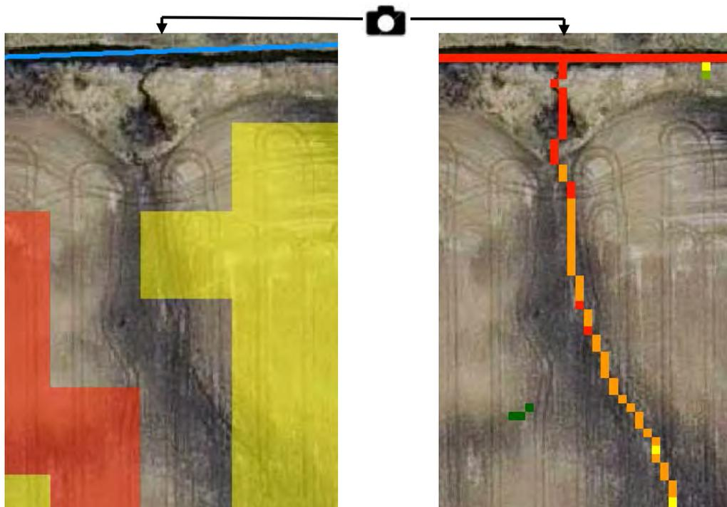
Observations and lessons learned: In ditched stream sections with steep, high walls, an SPI signature as short as one to two pixels (depending on threshold used) can often coincide with significant erosion in the field as compared to the same length signature along flat riparian areas. When using short SPI signatures to identify and rank potential CSAs, it is especially important to consider contributing area and soil erosion risk characteristics for each point.
