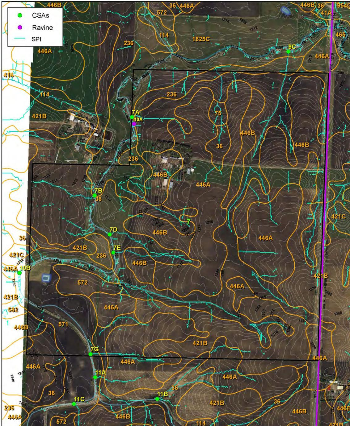
Site 7 did not initially have a CSA indicated on the map. The analyst saw the BMP (grassed waterway) in the aerial and did not place a CSA. The field survey indicated that there was significant stream bank erosion caused by the side inlet structure and that stream bank protection might be necessary. This finding resulted in the placement of a CSA when doing the terrain analysis despite that fact that an existing BMP was in place.
