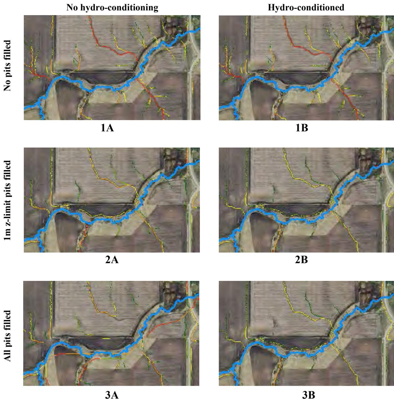
The above figures show SPI signatures calculated from a 3 meter DEM with varying degrees of pre-processing performed. All SPI signatures are from the 97.5<sup>th</sup> percentile within the extent shown (~136 acres). Figures in the left column were not hydro-conditioned, while figures in right column were – the DEM was hydro-conditioned by burning the stream (blue line) through the north-south oriented road crossing culvert in the top-right of image.
