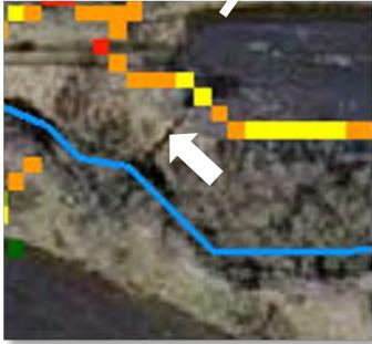
The first image (previous page) is an orthophoto taken in the spring of 2011 with several gullies evident, followed by the same photo with an SPI layer overlain (above). The SPI signatures closely match the surface erosion where flows concentrate. Note the white arrows highlight differences between apparent erosion on the photo vs SPI signatures, likely explained by the gap between date of LiDAR flown (11/27/2008) and aerial photo acquisition (mid-April, 2011).
