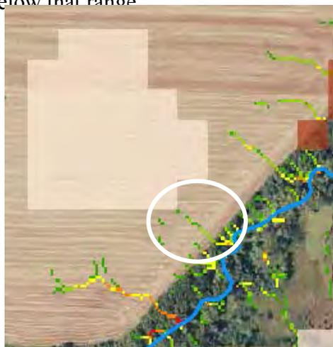
The image on left shows a series of small SPI signatures originating in an upland cultivated crop field. The large, tan colored shape represents the top 15% of the Soil Erosion Risk values (30 meter pixels) within the Pelican Lake HUC12 catchment (Stearns Co., MN). A field visit confirmed slight erosion occurring from the signature nearest the high Soil Erosion Risk percentile values (circled in white).
