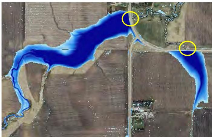
The left image shows an example of how water ponds (in blue) behind road crossings when using a non-conditioned DEM. There are culverts present at both crossings (circled in yellow), though the DEM does not recognize culverts and sees the road as an obstruction – known as a digital dam. Ideally all DEM’s used for SPI creation should be hydrologically corrected, though the process can be time consuming and small culverts may not show up in aerial photography making field verification necessary.
