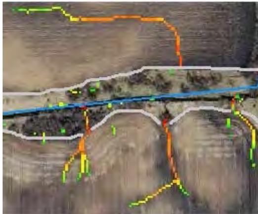
The grey horizontal lines represent the extent of the stream buffer. The top signature terminates at the buffer-field edge. The lower signatures terminate at the stream edge. *Note:* the bottom middle signature terminates just past the buffer. A field visit verified a steep knick point drop to water level at the signature terminus.
