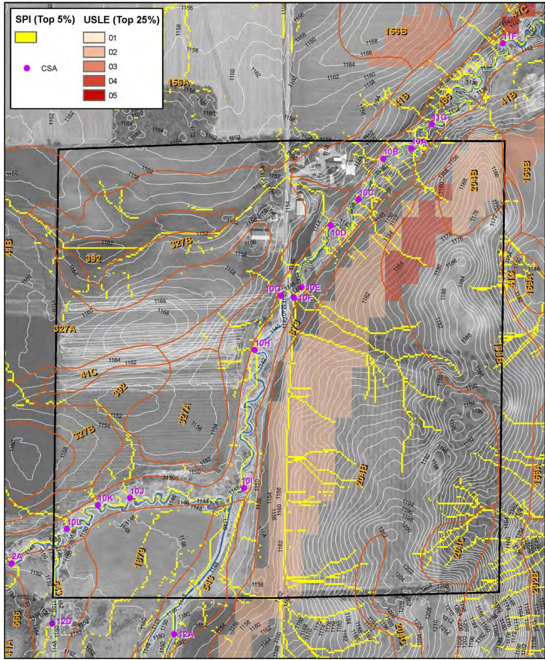
CSA 10H had a few SPI signatures converging on it and was a location where the meandering stream came very close to the field edge. When evaluated in the field no signs of channelization and very minimal signs of sedimentation were observed at the pour point. Good landuse management and a functional buffer were found at this site limiting the potential for issues at this CSA.
