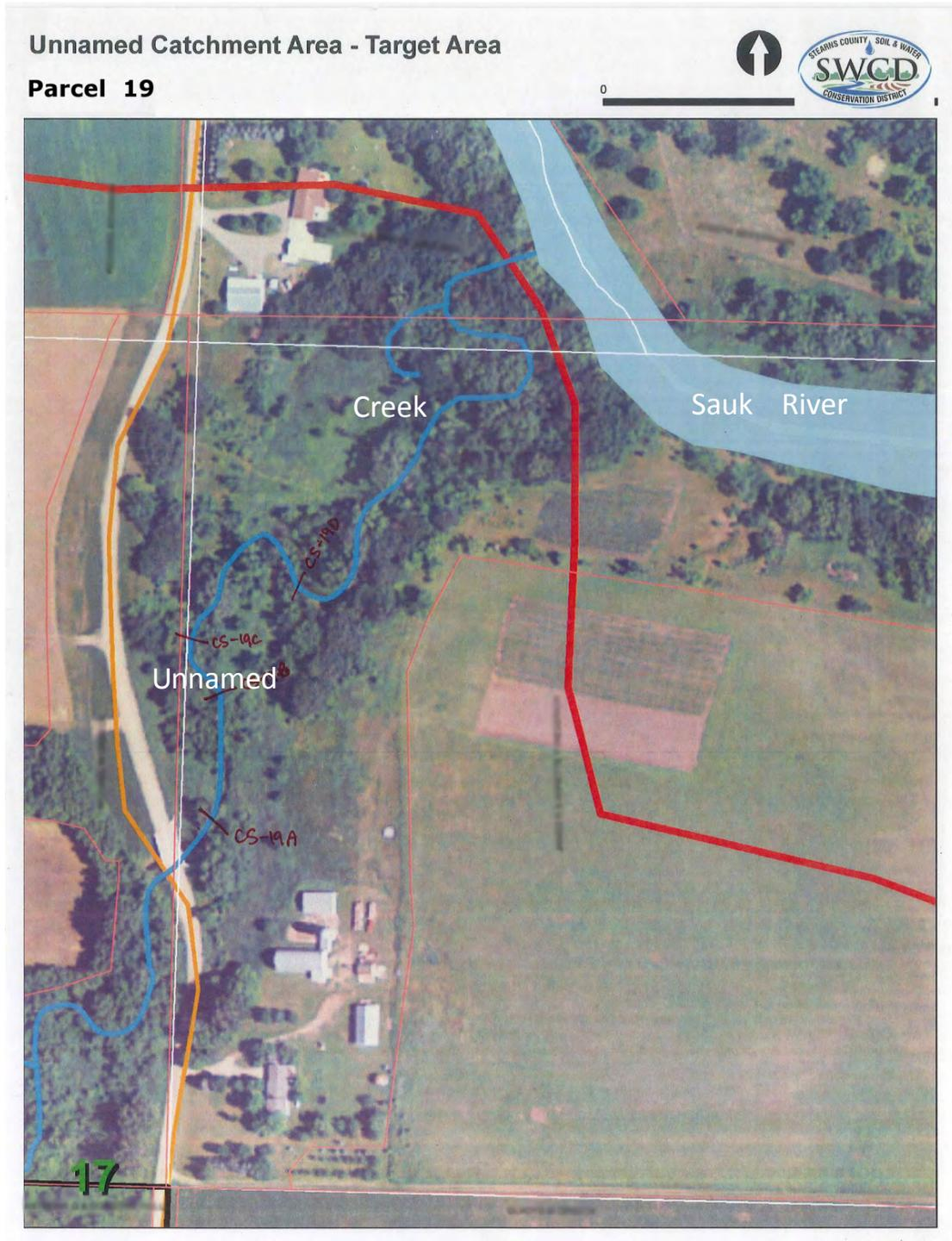
Although no CSA’s were present at Site 19, a number of the field tools were completed at selected cross sections along the channel. The BEHI determinations resulted in “moderate” to “high” ratings. The outside bends of this meandering stream exhibited poor root density, poor bank vegetation, and minimal access to the floodplain especially in wooded areas. The first site, Cross Section 19A, had a good buffer but a lack of access to the floodplain. The channel bed was full of fine eroded sediment.
