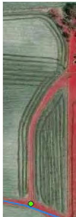
The three images, starting from the furthest left, show an SPI signature leading to an intermittent stream. The middle image shows conservation practices exist under the SPI signature, in this case a grassed waterway. Using CIR orthophotos, shown in the right image, can also greatly aid in detecting vegetated areas. CIR photos show vegetation as red and bare soil as green color.
