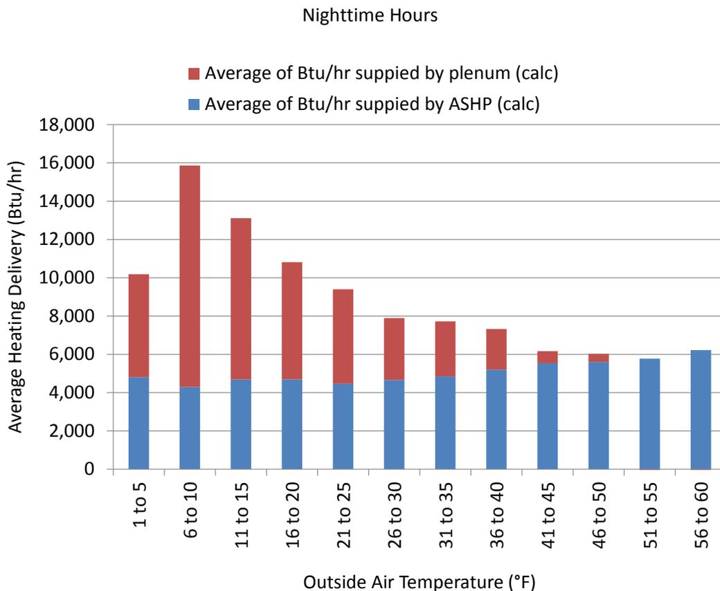
The controls in Home "A" are shown to allow for finer control of modulating electric heat across temperature ranges when compared to Home "N". As Figure 15 illustrates, the plenum heater contribution to Home "N" is more stepwise (increasing significantly below 20° F), showing the system is
