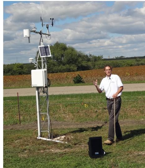
MDA staff, Luke Stuewe, in front of a recently installed weather station located at the Rosholt Farm in Westport, Minnesota. Weather information such as precipitation, air temperature, and wind speed can help local farmers plan their water and nitrogen management.
