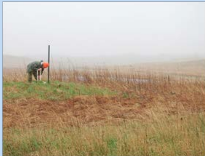
BWSR Hydrologist Eric Mohring installs data loggers at the site to track water levels.
