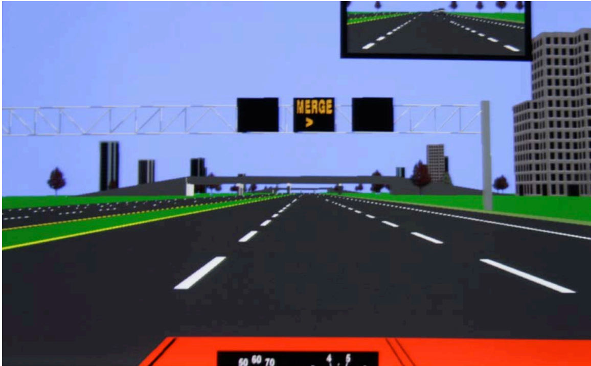
Figure 2.7 The fourth set of ILCSs with the first in the sequence of dynamic chevrons indicating merge right
