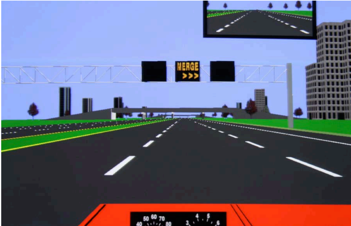
Figure 2.9 The fourth set of ILCs with the third in the sequence of dynamic chevrons indicating merge right
