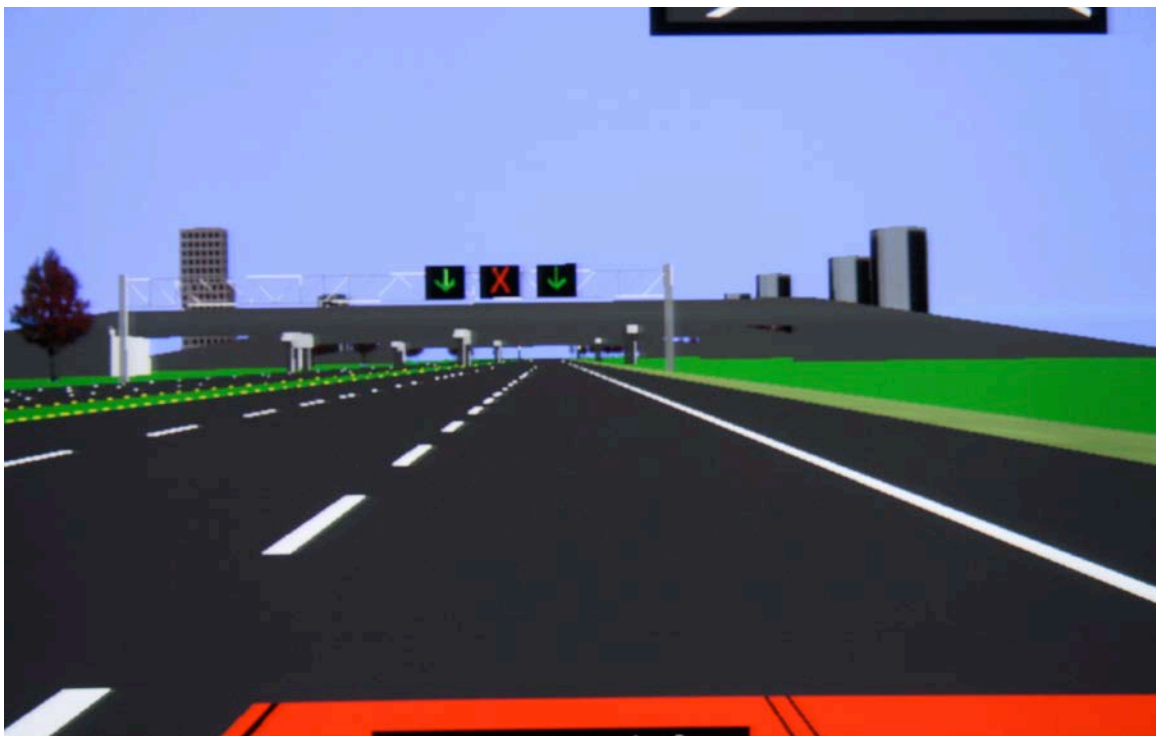
Figure 2.10 The fifth set of ILCs with the “X/1 mile” lane closure warning on the center display and green arrows on the left and right ILCs
