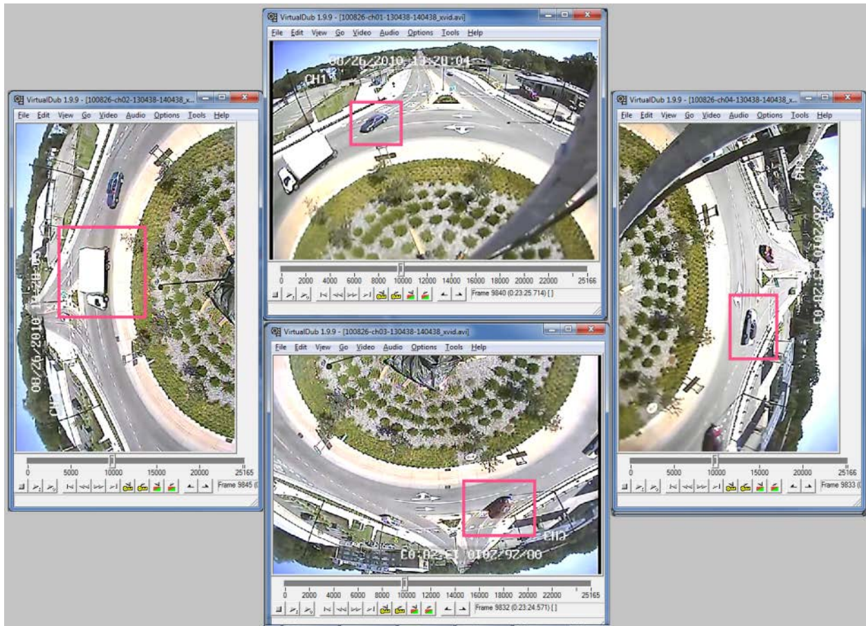
Figure 4-8 Estimation of Vehicle Density inside the Roundabout through Vehicle Count
