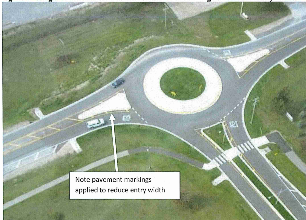
Figure 1 - Single Lane Roundabout with Pavement Markings to Reduce Entry Width
