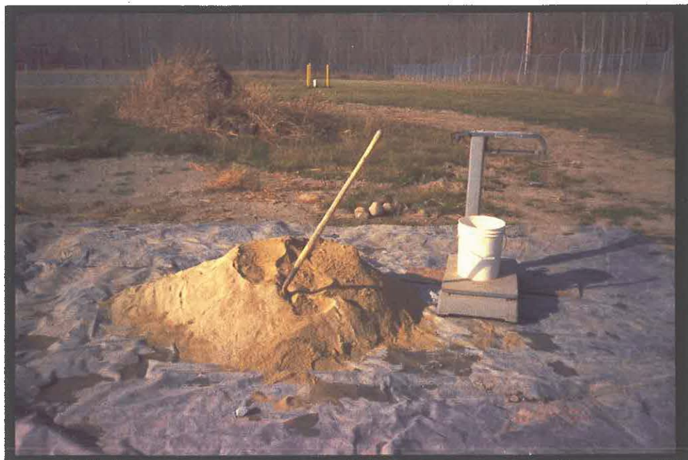
Figure 4. Limestone used for the alkaline mixture experiment. The limestone product was purchased from Aggregate Resources' Larson Mine on Grey Cloud Island and is called a manufactured sand.
