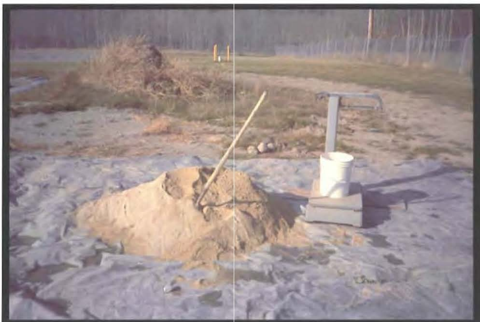
Figure 13. Limestone used for the alkaline mixture experiment. The limestone product was purchased from Agrrerate Resources' Larson Mine on Grey Cloud Island and is called a manufactured sand
