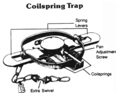
Coil-spring traps are the fastest of the foot hold traps. Available in sizes 1 through 4 from a variety of manufacturers, coil springs are often used in trapping predators. They have all the advantage of under-spring traps with the addition of increased speed.
