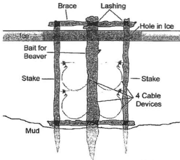
Cable devices can also be set as live-restraining traps in water and anchored on land. This will allow the furbearer to leave the water.
