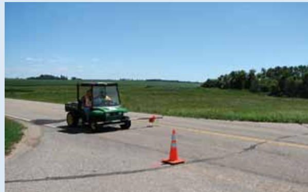
The new combined pavement specification is based on data from inertial profilers like this one, which use laser sensors to take precise measurements of smoothness.
