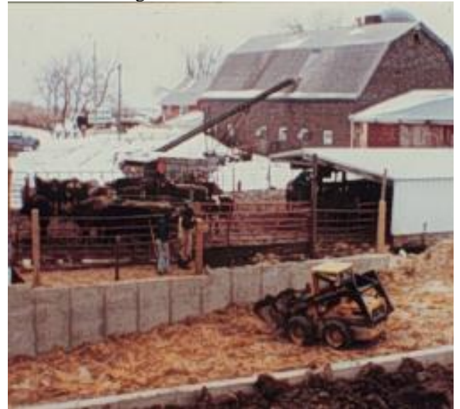
Figure 4. Typical scrape and haul manure management with skidsteer loader
