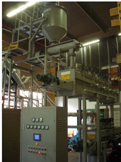
Figure 3. Large pilot microwave assisted pyrolysis system installed at the Center for Biorefining, University of Minnesota.
