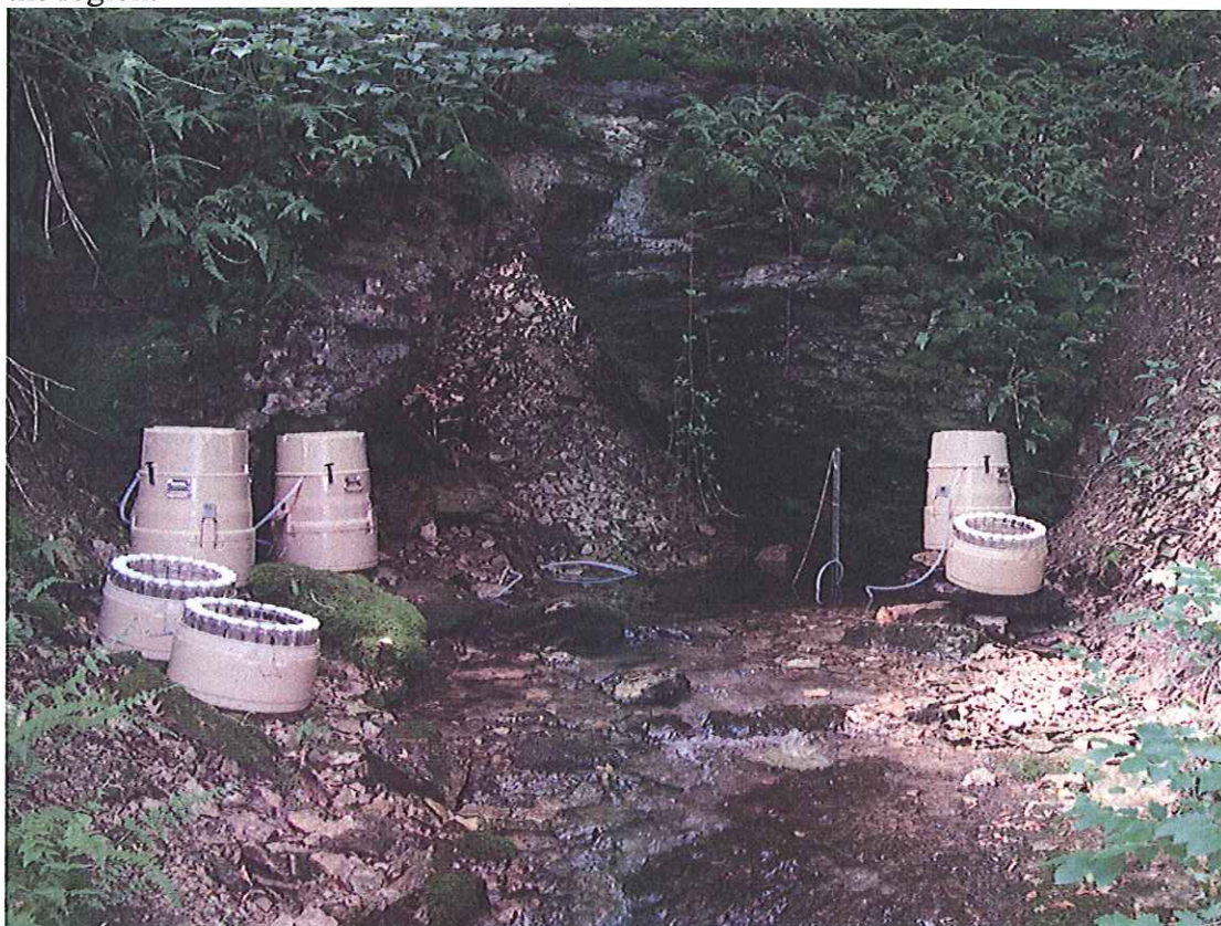
Fig. 1. Bat River Spring with ISCO 3700 auto samplers in place
