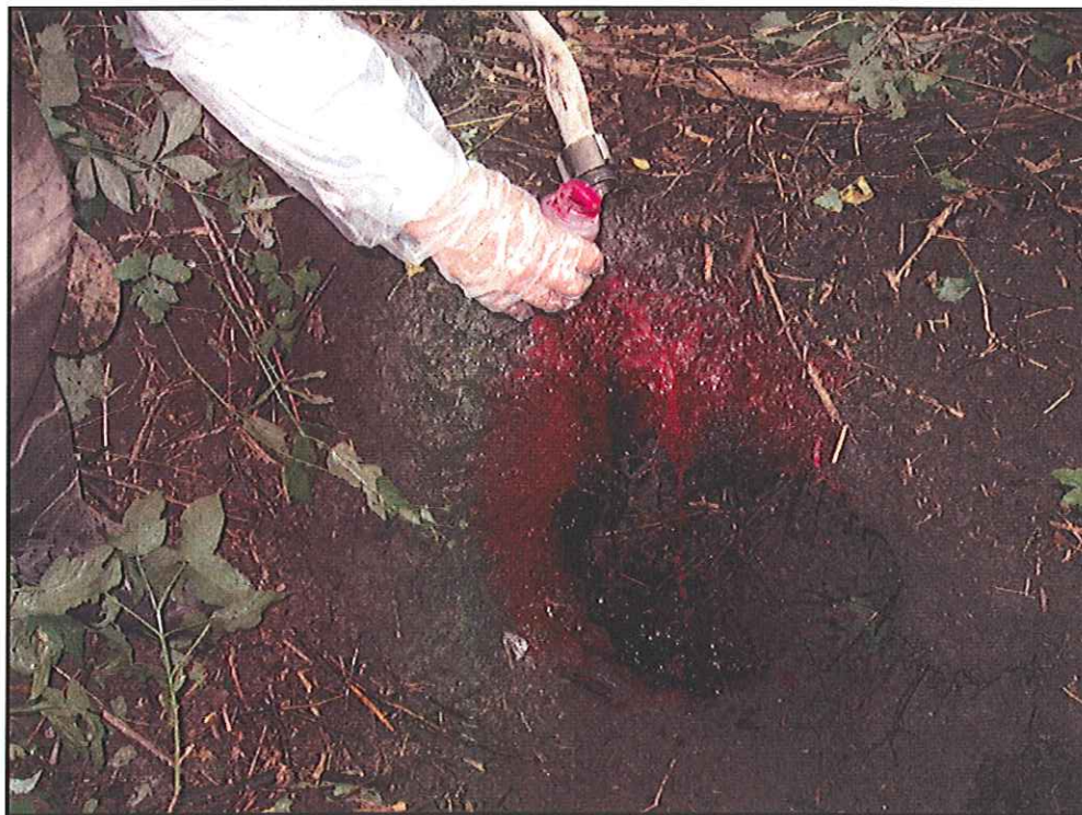
Figure 11. Introduction of sulforhodamine B to sinkhole D162.
