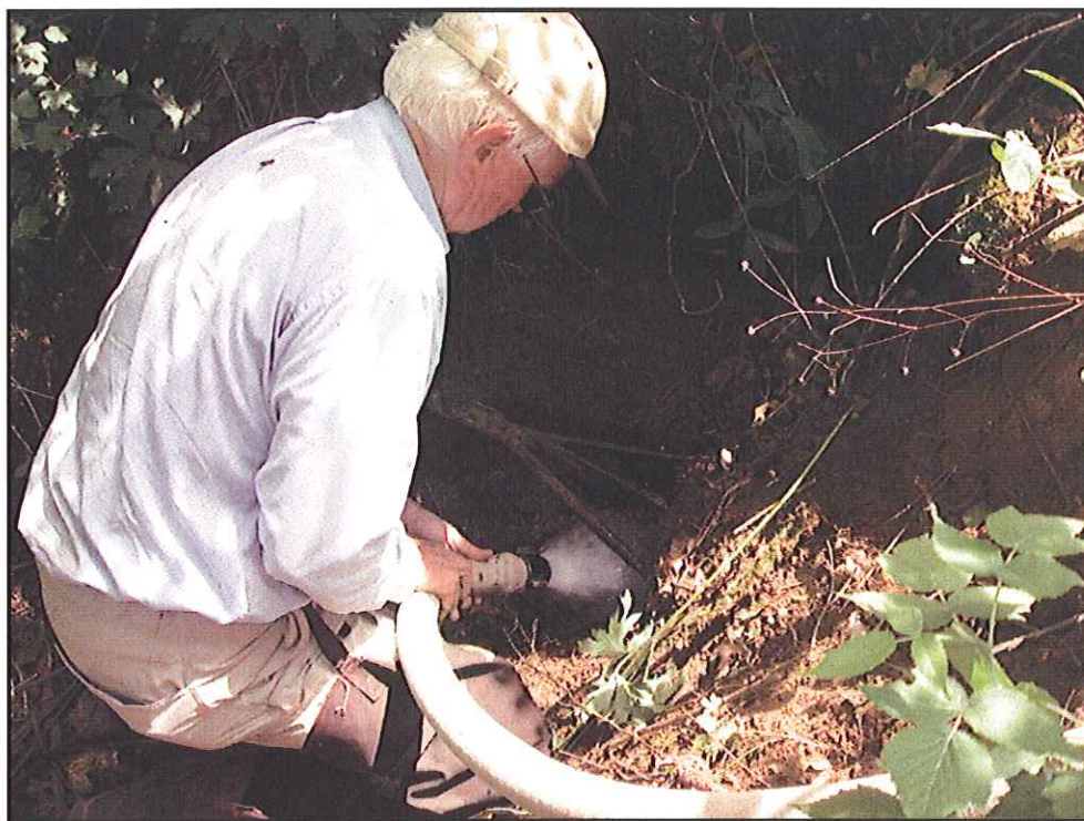
Figure 12. Calvin Alexander introducing water and eosine dye into sinkhole D133.
