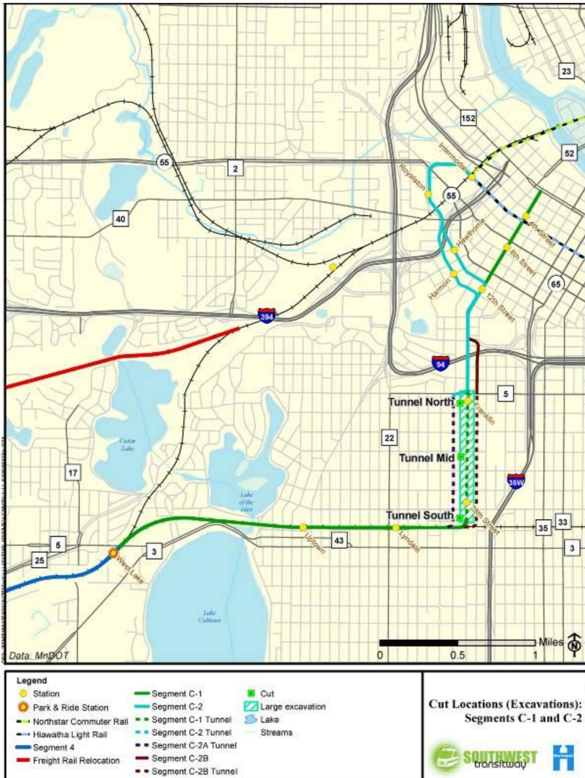
Figure 4. Cut Locations (Excavations): Segments C-1 and C-2
