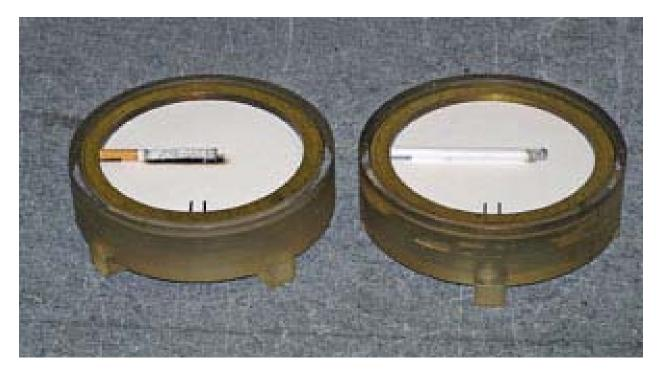
Note: The photo above is provided for illustration purposes only. It is not intended to represent the complete application of the ASTM Standard E2187-04 testing process as it would be performed in a laboratory.
