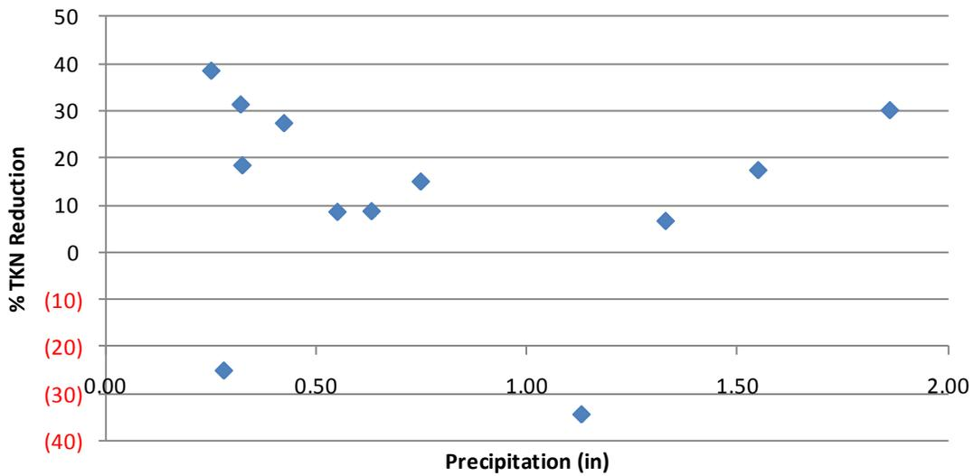
**Figure 40. Platteville Buffer: Reduction of TKN as a function of precipitation.**
