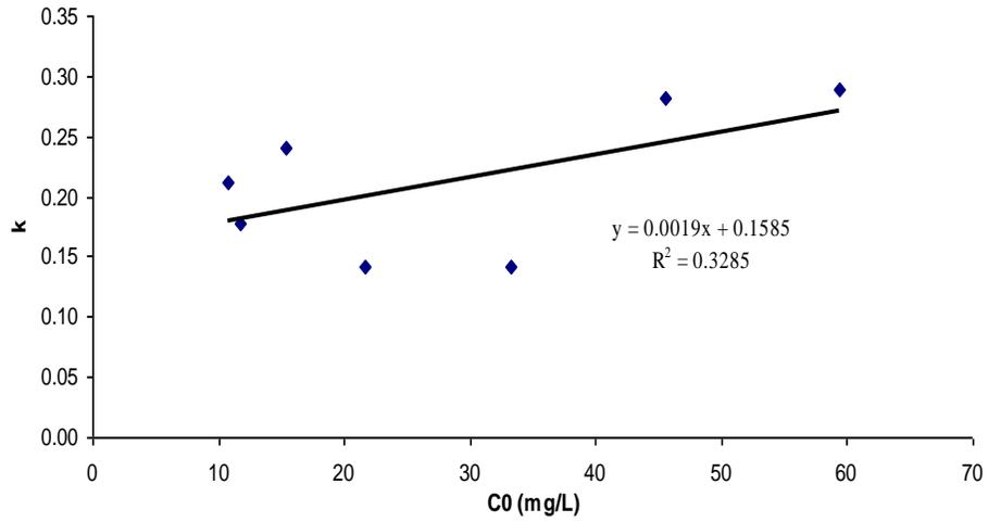
**Figure 47.  $k$  vs.  $C_0$  for the first-order model of P**
