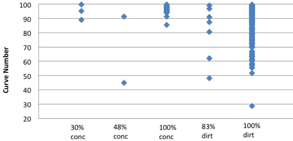
**Figure 2. Variation in Curve Numbers with Feedlot Type (conc =Concrete).**
