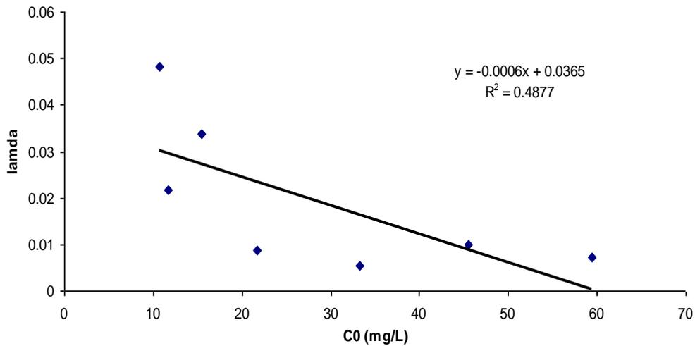
**Figure 49.  $\lambda$  vs.  $C_0$  for the logistic model of P**
