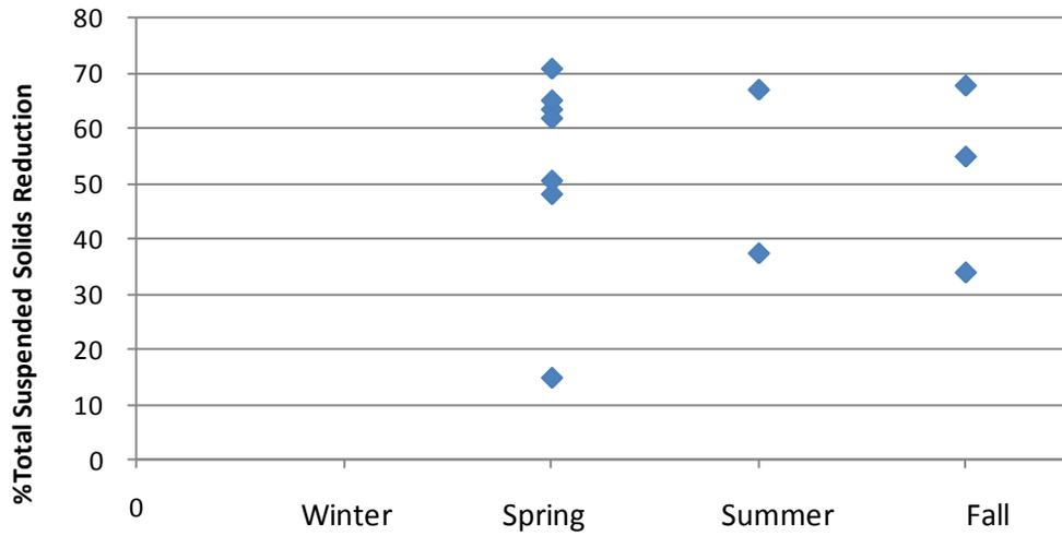
**Figure 35. Platteville Buffer: Reduction in Total Suspended Solids Concentration as a function of Season.**
