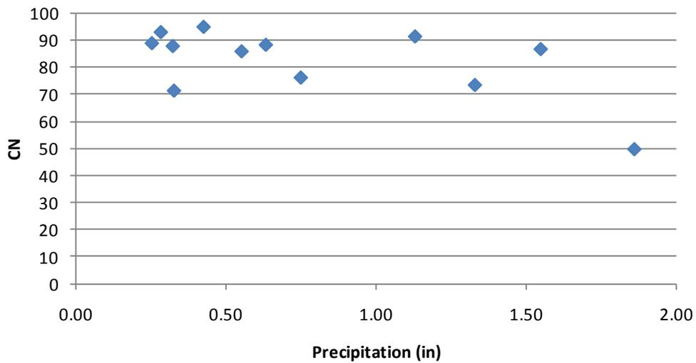
**Figure 32. Platteville Buffer: Curve Number as a function of Precipitation.**
