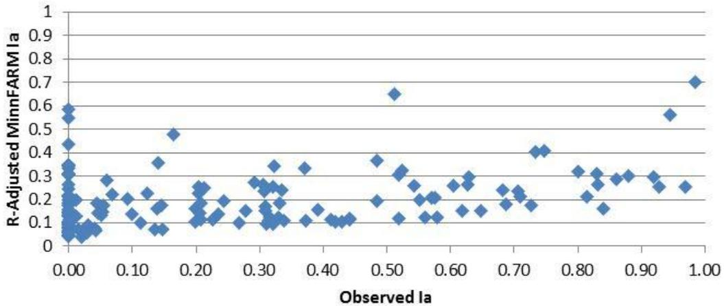
**Figure 17. Recommended MinnFARM Predicted and Observed  $I_a$  for  $P < 1$  inch.**
