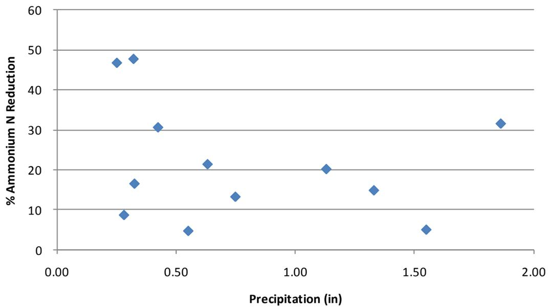
**Figure 37. Platteville Buffer: Reduction of Ammonium-N as a function of Precipitation**
