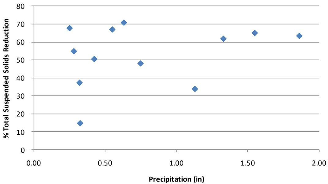
**Figure 36. Platteville Buffer: Reduction in Total suspended Solids Concentration as a function of Precipitation.**
