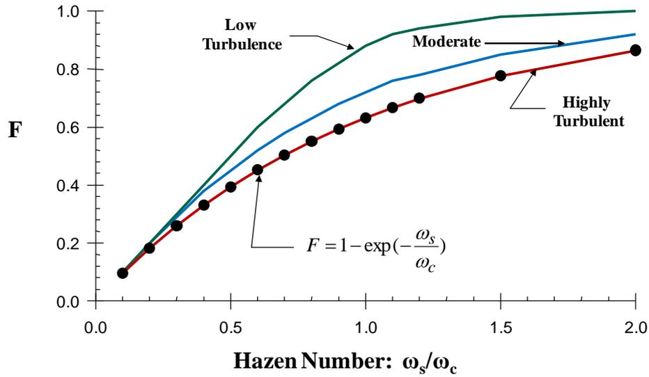
**Figure 45. General Solution for Removal Efficiency in Settling Chamber**
