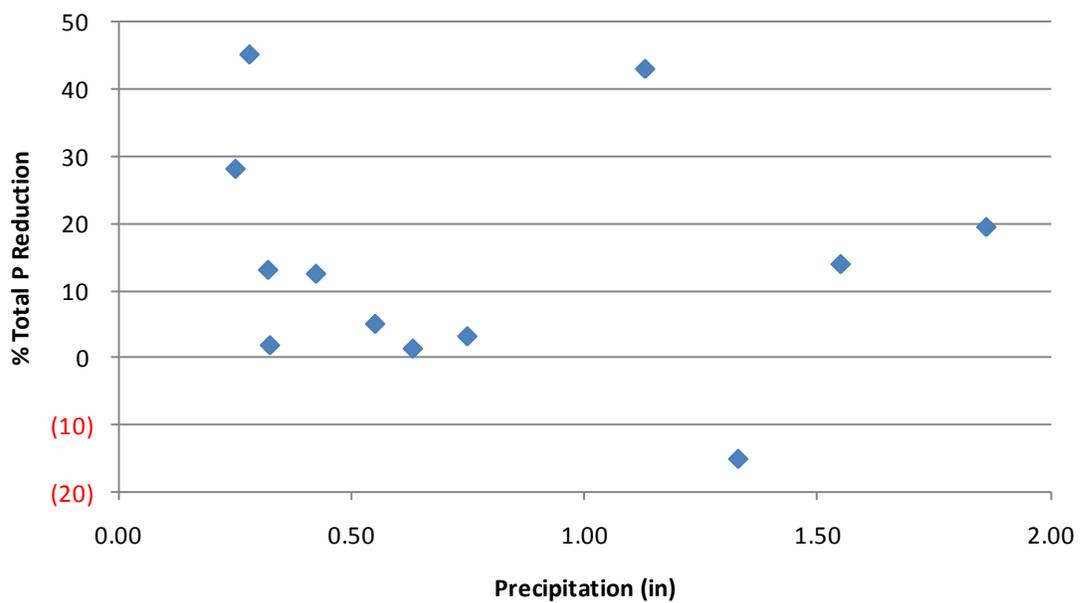
**Figure 41. Platteville Buffer: Reduction of Total P as a function of precipitation.**
