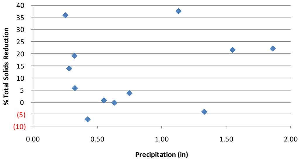
**Figure 34. Platteville Buffer: Reduction in Total Solids Concentration as a function of Precipitation.**
