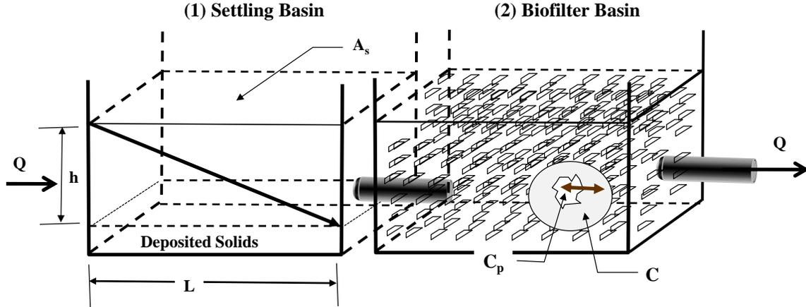
**Figure 44. Schematic of the biofiltration system.**
