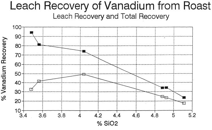
Data from Magnetic Separtator and Flotation Concentrates
