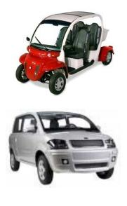
The electric vehicles are rechargeable through the electrical grid and have a range of between 30 to 75 miles before needing to recharge. Models come in styles ranging from two-seaters to small-scale trucks, normally weighing between 1,000 and 1,500 pounds. Originally produced mostly for niche uses such as military bases and planned communities, their use has widened. The largest U.S. market is in California.
