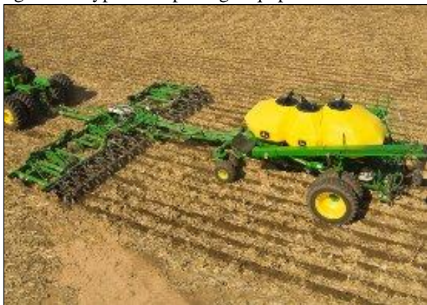
Figure 7. Typical strip tillage equipment
