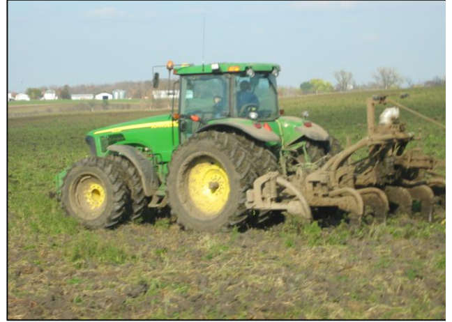
Figure 2. Umbilical manure application equipment used in Carver County
