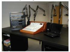
fashion, so as to make it possible to easily relocate it if necessary. The studio has a six-channel audio mixer, two CD players and an automation system. There are five microphones: the announcer mic and four guest mics. This studio can operate independently from KMSU, or can be the source for both KMSU and KMSK. This is the station's first step towards providing truly local arts and cultural programming for the Austin community rather than relying on having everything come out of Mankato.
