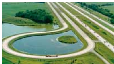
The MnROAD test facility, which is promoted by TERRA through pooled fund study TPF-5(215), consists of 3.5 miles of working interstate freeway and a 2.5-mile closed loop for low-volume traffic to simulate rural road conditions. These pavements are equipped with electronic sensors to support a wide range of tests to investigate new pavement construction methods and materials.
