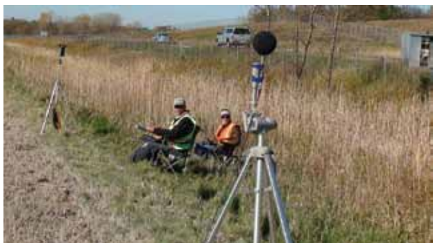
In Report 2010-40, "Influence of Pavement on Traffic Noise—Statistical Pass-By Measurements of Traffic on Several Interstate Pavements," investigators monitored pavement noise for test sections using microphones placed at distances of 100 feet, 500 feet and directly adjacent to the road.
