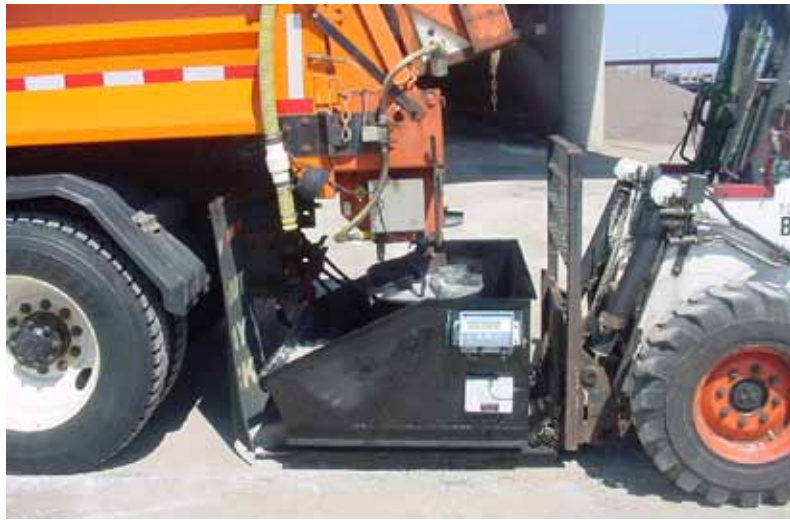
The weight box shown here is a simple-to-use tool that automatically weighs material for sander calibration. The weight box can collect approximately 500 pounds and requires a skid steer or forklift for positioning and emptying.
