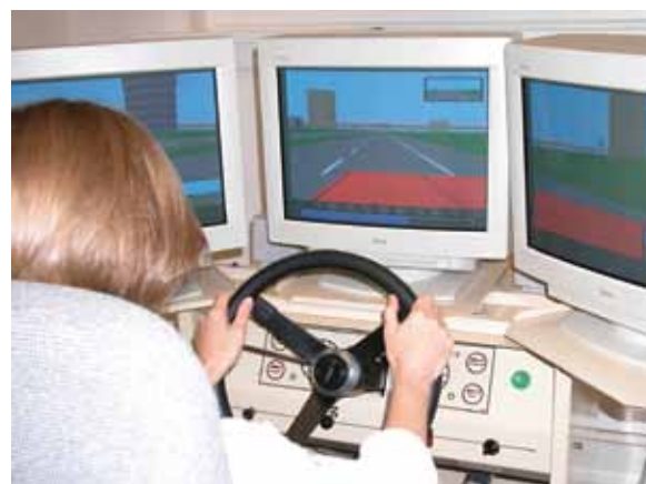
In Report 2010-02, “ Comparison of Dual-Phase and Static Changeable Message Signs to Convey Airline Information on Interstate Freeways, ” researchers used a driving simulator to compare the use of overhead dual-phase to multiple static Changeable Message Signs for effectiveness in conveying airline information to drivers approaching the Minneapolis-St. Paul International Airport by highway.
